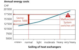
Annual energy costs of a system with (evaporator) power of 210 kW with different degrees of soiling of heat exchangers.
