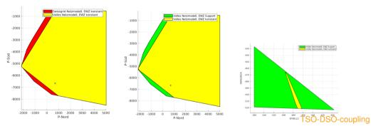
limits the available range. Without coupling risk of unsecure grid states. The flexibility can be recovered with DSO-support via the trafo settings.
