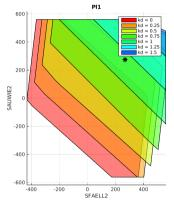
DSO grid: Available trafo capacity and operating surface for different loads
