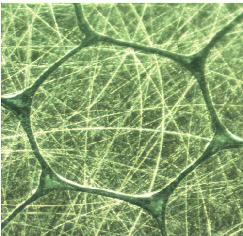
The microscopic image shows the cross-section of a single strand of a stator winding: The strand takes on a hexagonal shape because of mechanical shaping. Photo: BRUSA
