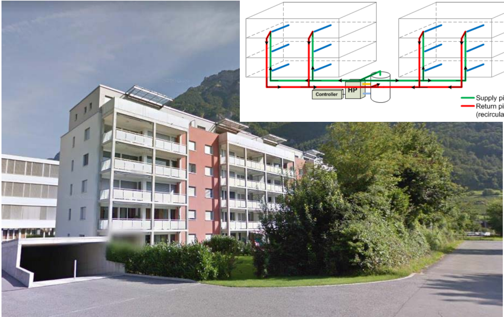
Conventional recirculation implemented in reference building
