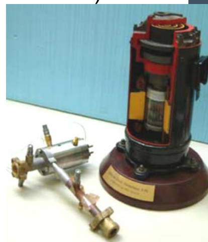
Size comparison (Turbo vs. Scroll compressor)
