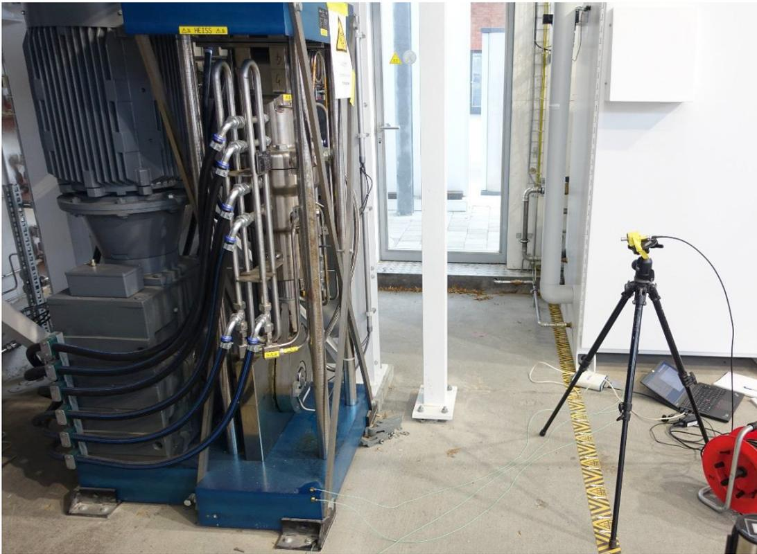
The compression of hydrogen to 700 bar produces noise that can affect the neighborhood. This noise can be shielded through a suitable sound insulation device. In the picture right: a device for sound measurement. Photo: Prose
