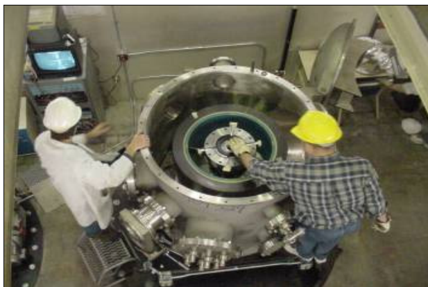
Figure 1: Testing a prototype of an HTSC flywheel developed by Boeing (source: Boeing, USA)
