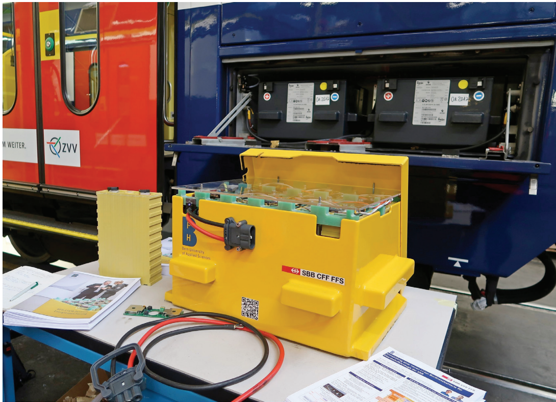
Presentation of the functional prototype at the Association of Public Transport (VÖV). In the background, a regional train wagon DPZ outfitted with lead-acid batteries, which are being phased out. Photo: SBB
