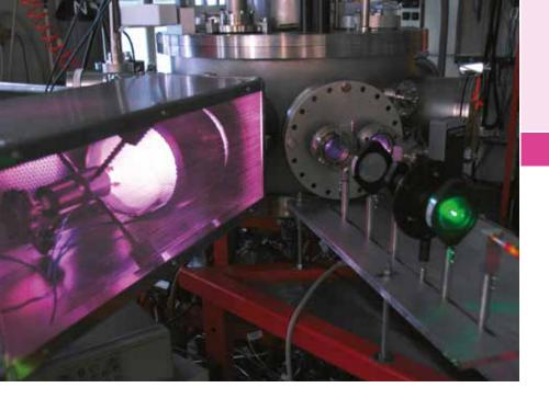
Development of reflectors for the ITER experimental reactor: Left (purple): Plasma source for simulating the conditions for particle irradiation. Right (green): Light source for the simultaneous measurement of the reflection properties of the reflector.
