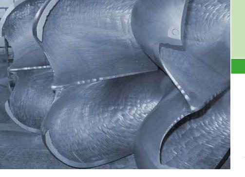
Abrasion damage on a Pelton wheel caused by a high content of suspended matter in the water intake.
