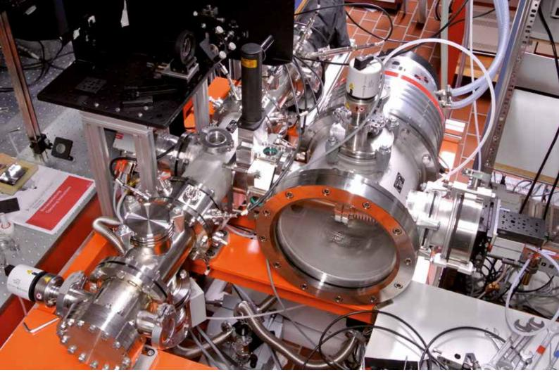
Experimental set-up for photoelectron spectroscopy at the Paul Scherrer Institute laser laboratory.
