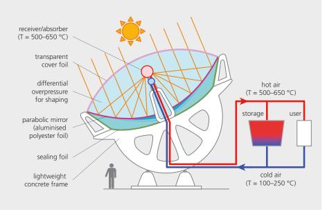
Solar parabolic trough concentrator developed by Airlight Energy, with pneumatic reflector comprising an aluminised polyester foil that is enclosed with a transparent cover foil. Air is used as the absorber medium.
