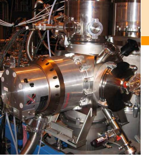
Experimental set-up at the Paul Scherrer Institute for spectroscopic coincidence measurements of photoelectrons and ions using the Swiss Light Source (synchrotron source). The purpose of these studies is to determine the thermo-chemical properties of combustion-relevant molecules in order to obtain data for more accurate simulations of complex combustion processes.
