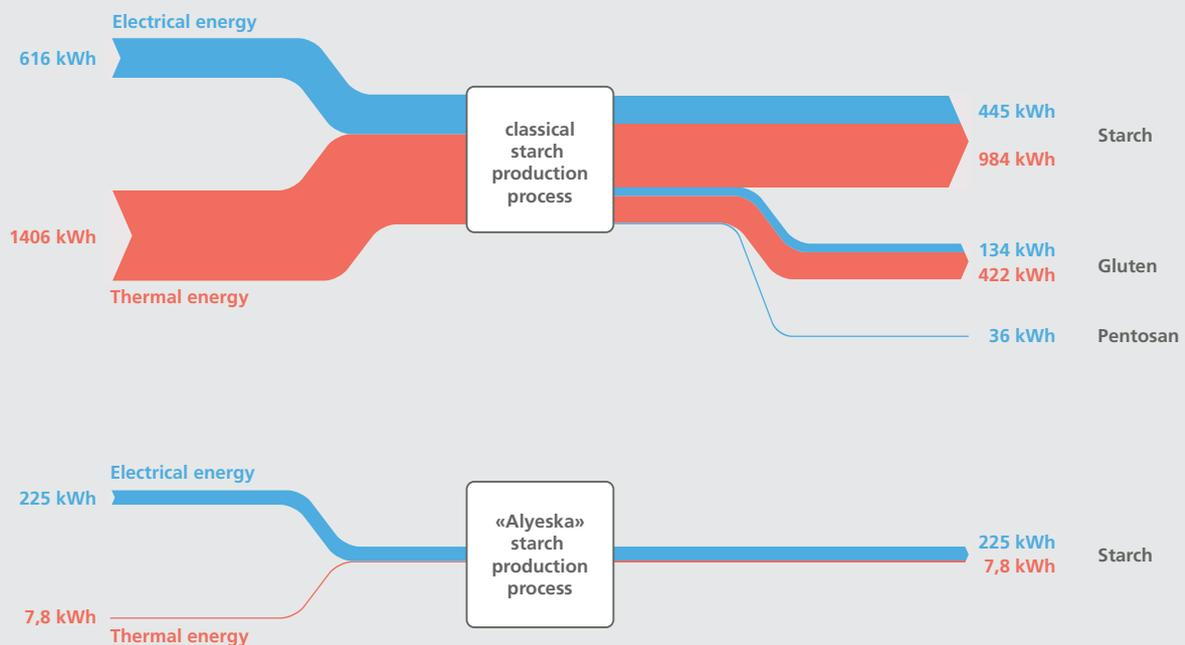
Sankey diagram relating to one tonne of starch product: the innovative “Alyeska” process for starch production requires significantly less heat (red) and electricity (blue) than the conventional starch production process.
