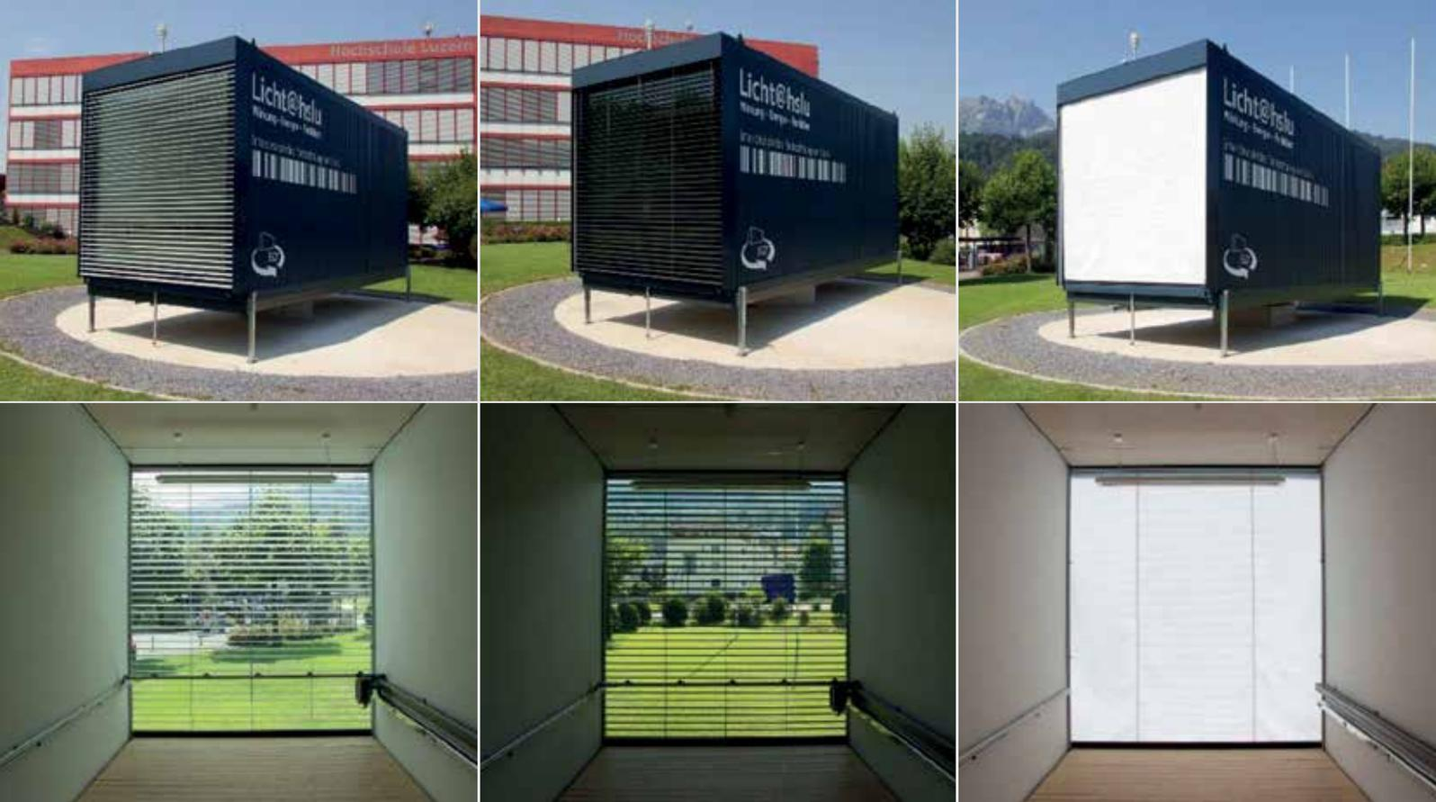
Container for measuring daylight illuminance set up at the Lucerne University of Applied Sciences and Arts in Horw: view of exterior (above) and interior (below).
