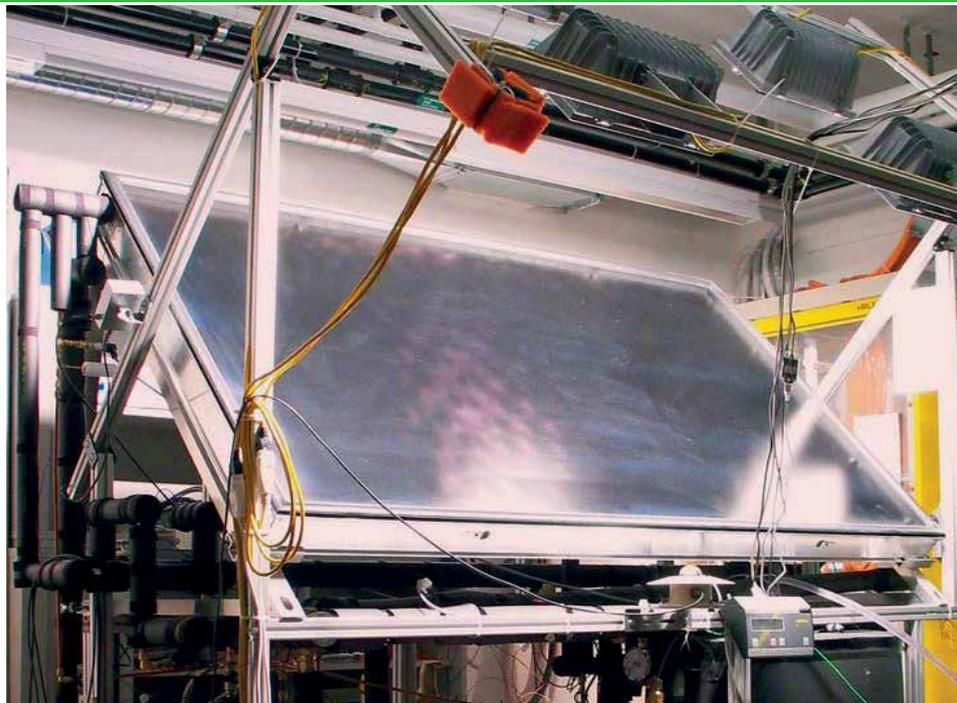
*At the Federal Institute of Technology, Zurich, a new low-cost method for the solar thermal degasification of hydraulic circuits was developed and patented. Its feasibility was demonstrated on a test bench set up specifically for this purpose.*
