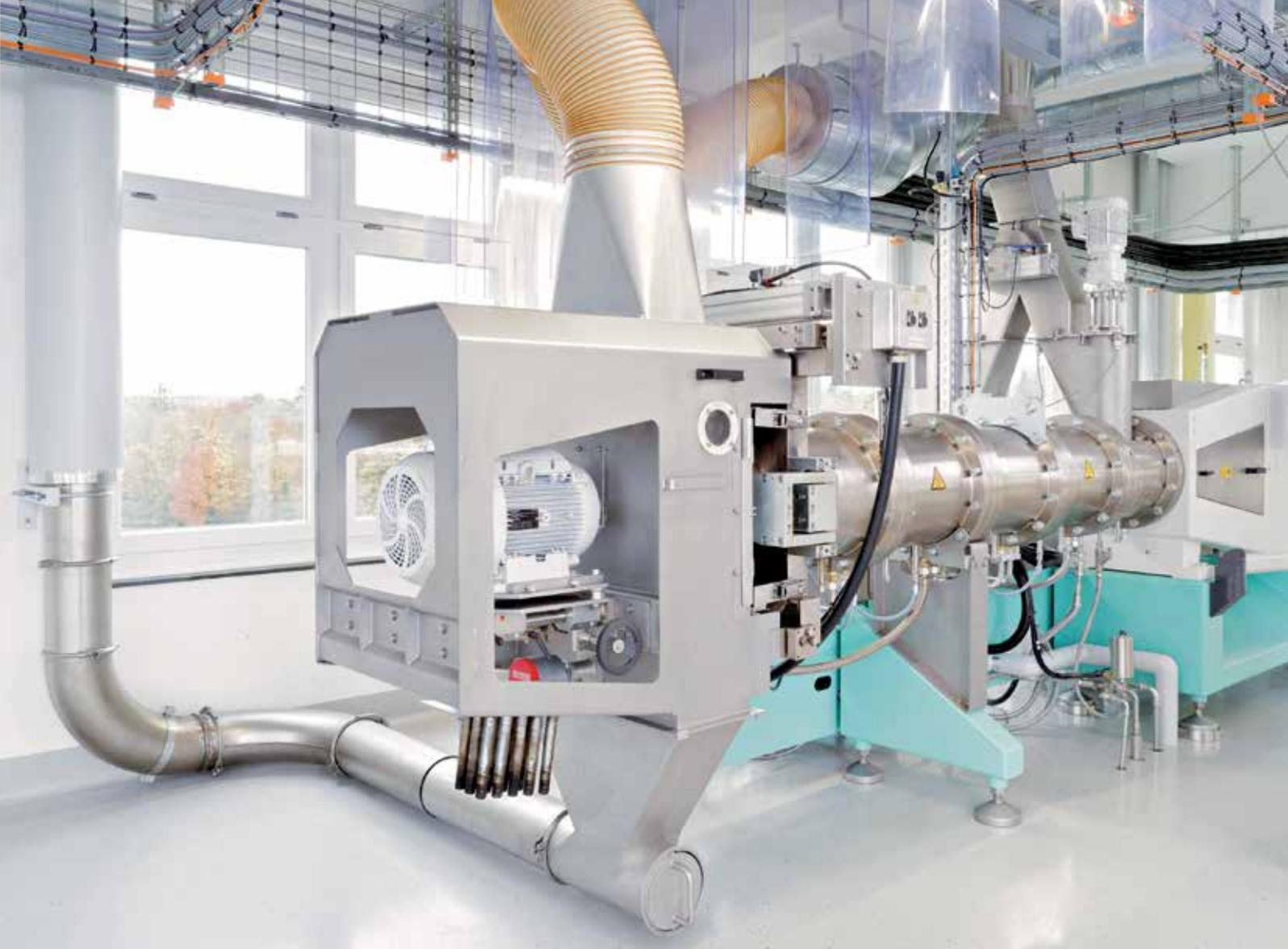
*An extruder is the central component in the new facility at Meyerhans Mühlen AG for the production of starch for use by the papermaking industry.*
