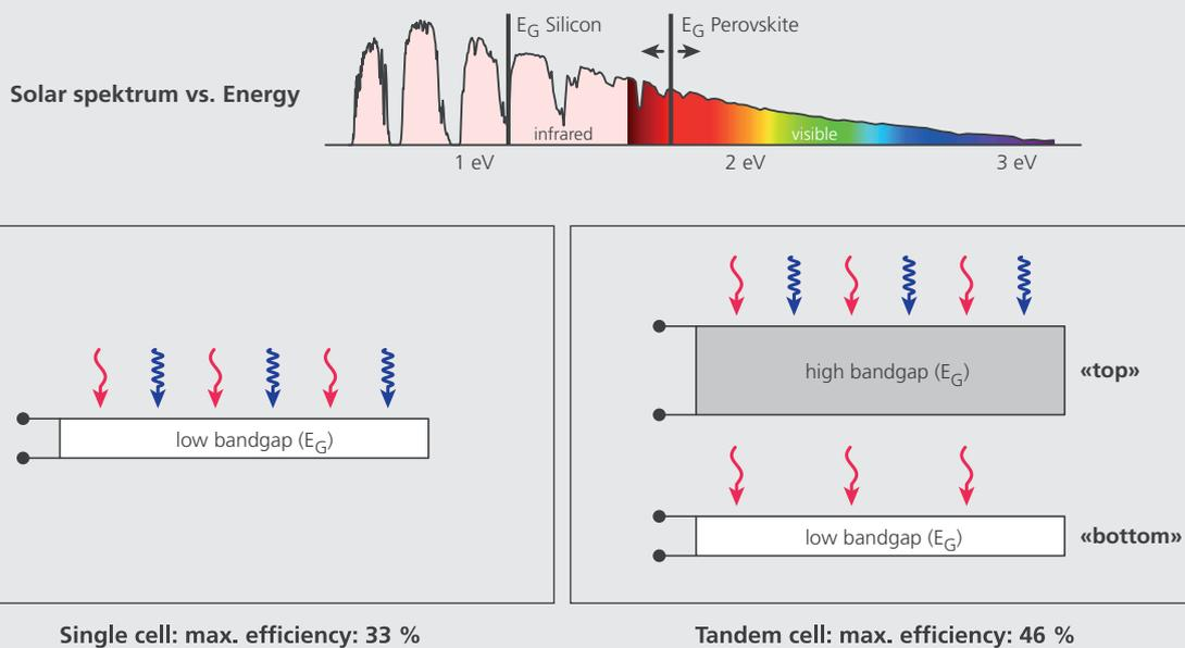
*Single cells with one absorber (left) can only use the portion of the solar spectrum with energy larger than the band gap of the specific semiconductor material. Light with a "too high" energy level is transformed into heat. In a tandem cell (right), materials with differing band gaps are stacked so that the top cell absorbs in the blue range. The red light is transmitted and absorbed by the bottom cell.*
