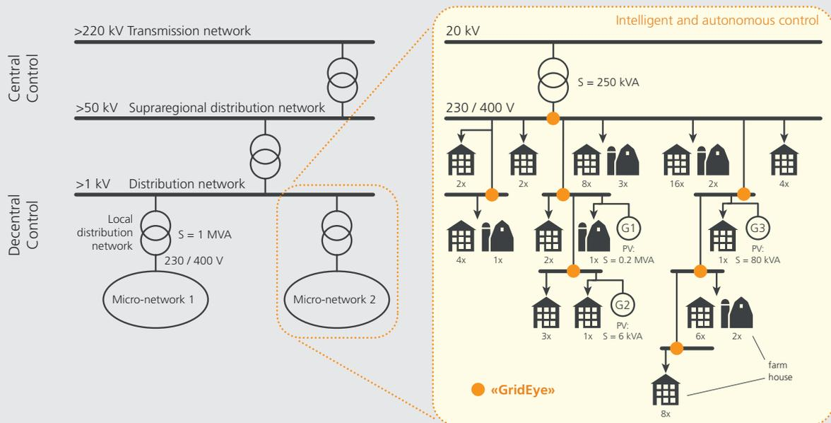
**The “GridEye” system measures voltage at grid points in the distribution network and enables the optimum operation of the grid via a smart and autonomous control system.**
