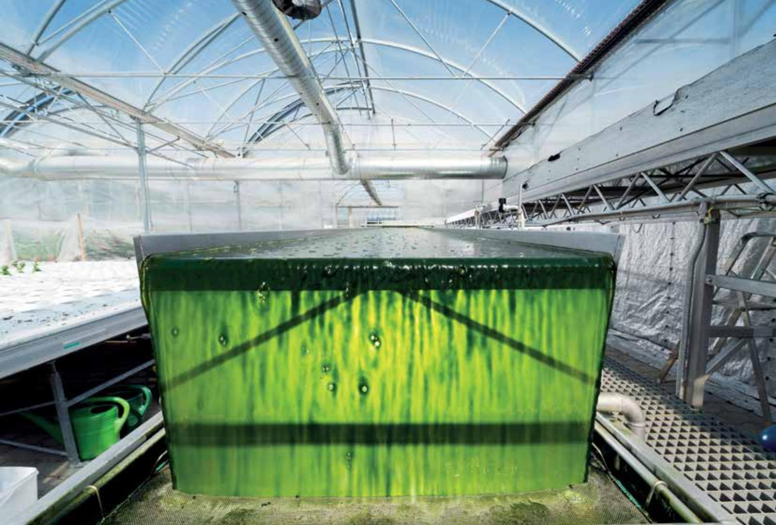
*Production of "Chlorella vulgaris" blue-green algae in an open thin-film photo-bioreactor at the Zurich University of Applied Sciences (ZHAW).*
