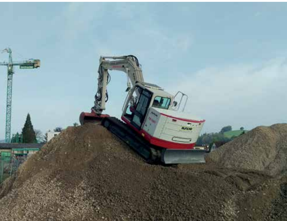
Prototype of an electric digger at work on a building site. The battery is situated in the raised structure at the rear, thus replacing part of the counterweight (image source: SUNCAR HK AG).
