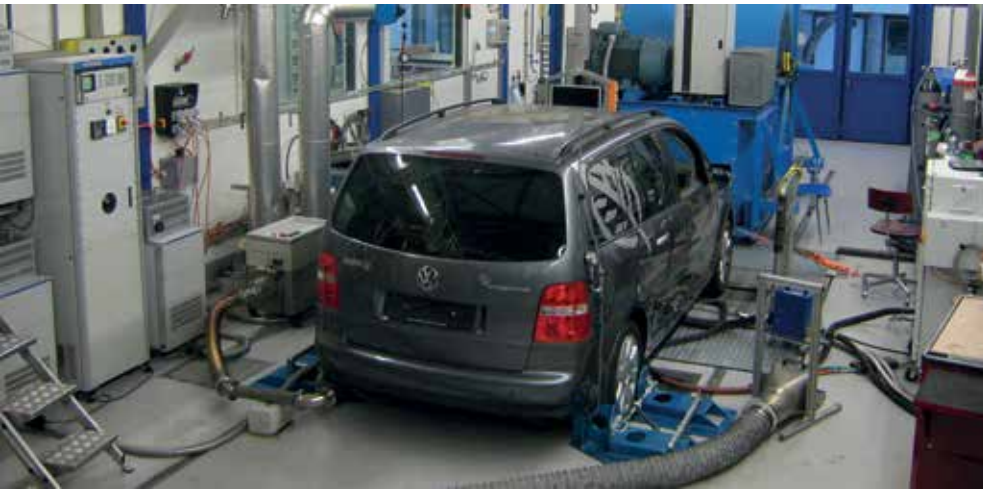
Measurement campaign on a Empa's roller test bench on a gas powered vehicle fuelled with natural gas enriched with hydrogen (image source: Empa).
