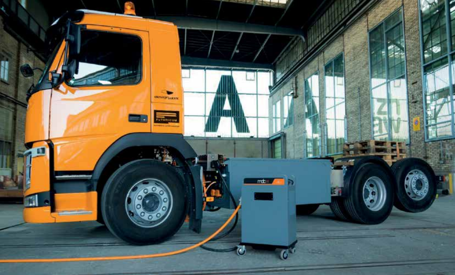
A newly developed 26-tonne electric truck prior to the refuse unit being installed. The large storage battery is situated between the wheel axles (image source: Designwerk).
