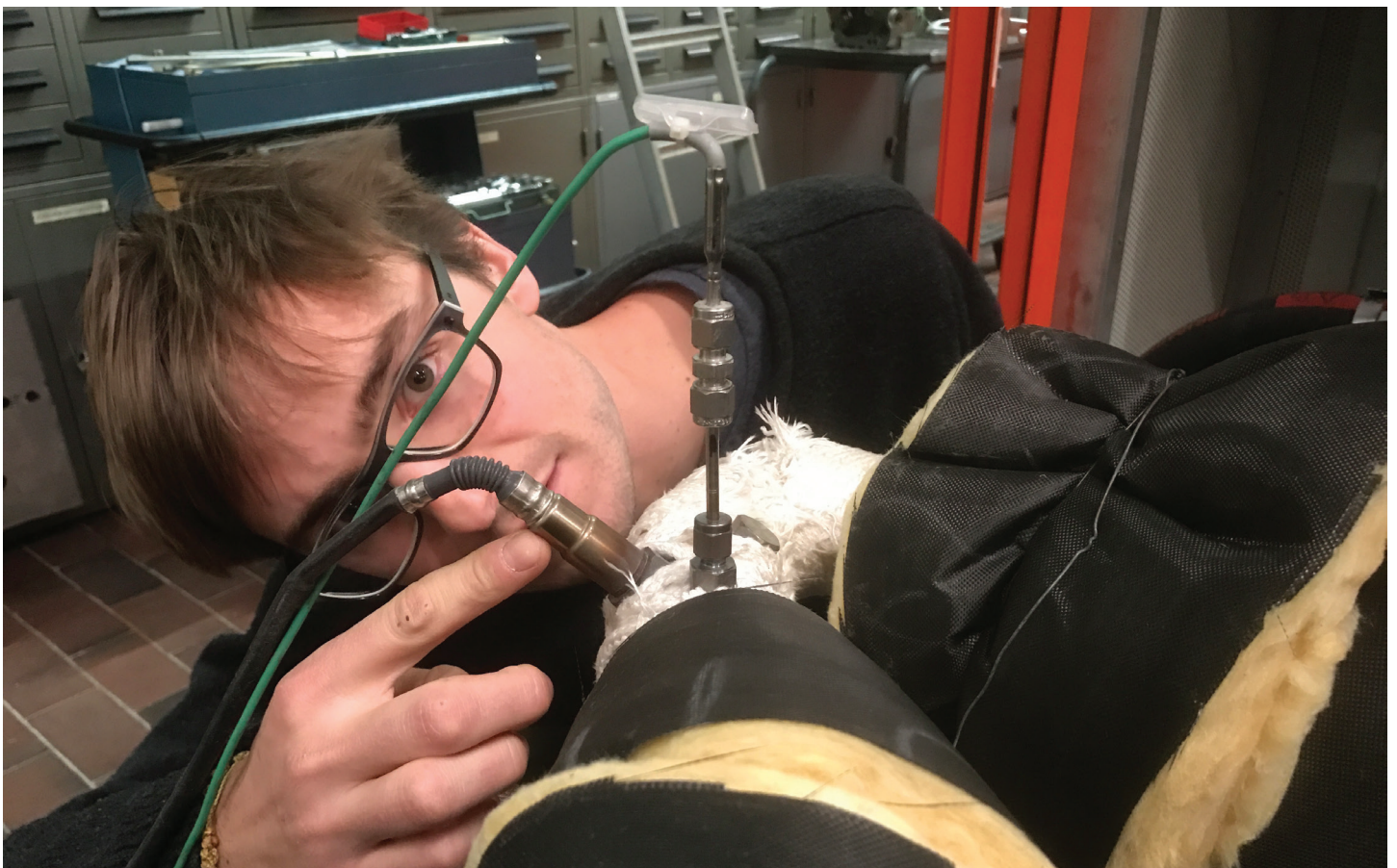
ETH researcher Christian Schürch with the laboratory model of the Micro-CHP. His finger points to the Lambda probe, to the right of it a temperature sensor for measuring exhaust gas temperature. Photo: B. Vogel
