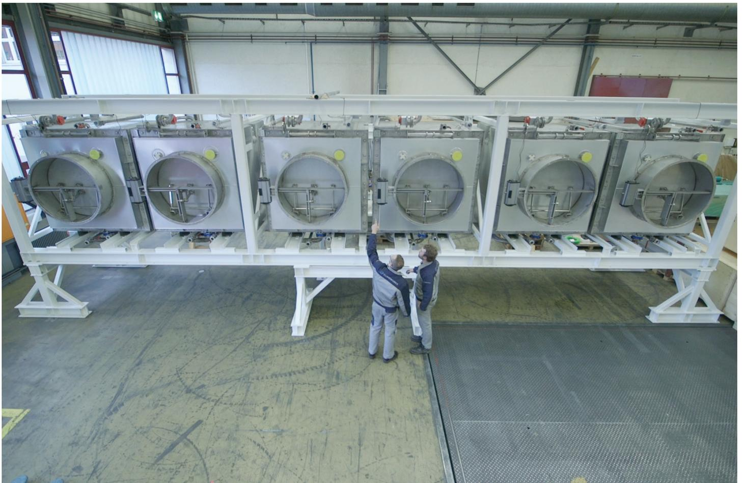
Six modules for CO<sub>2</sub> capture are housed in a 40-foot shipcontainer. They are located at Climeworks company headquarters in Zurich-Oerlikon, ready to be installed at the pilot and demonstration facility in Hinwil in the Zurich Oberland region. The facility for CO<sub>2</sub> capture shall go in operation in spring 2017. Photo: Climeworks
