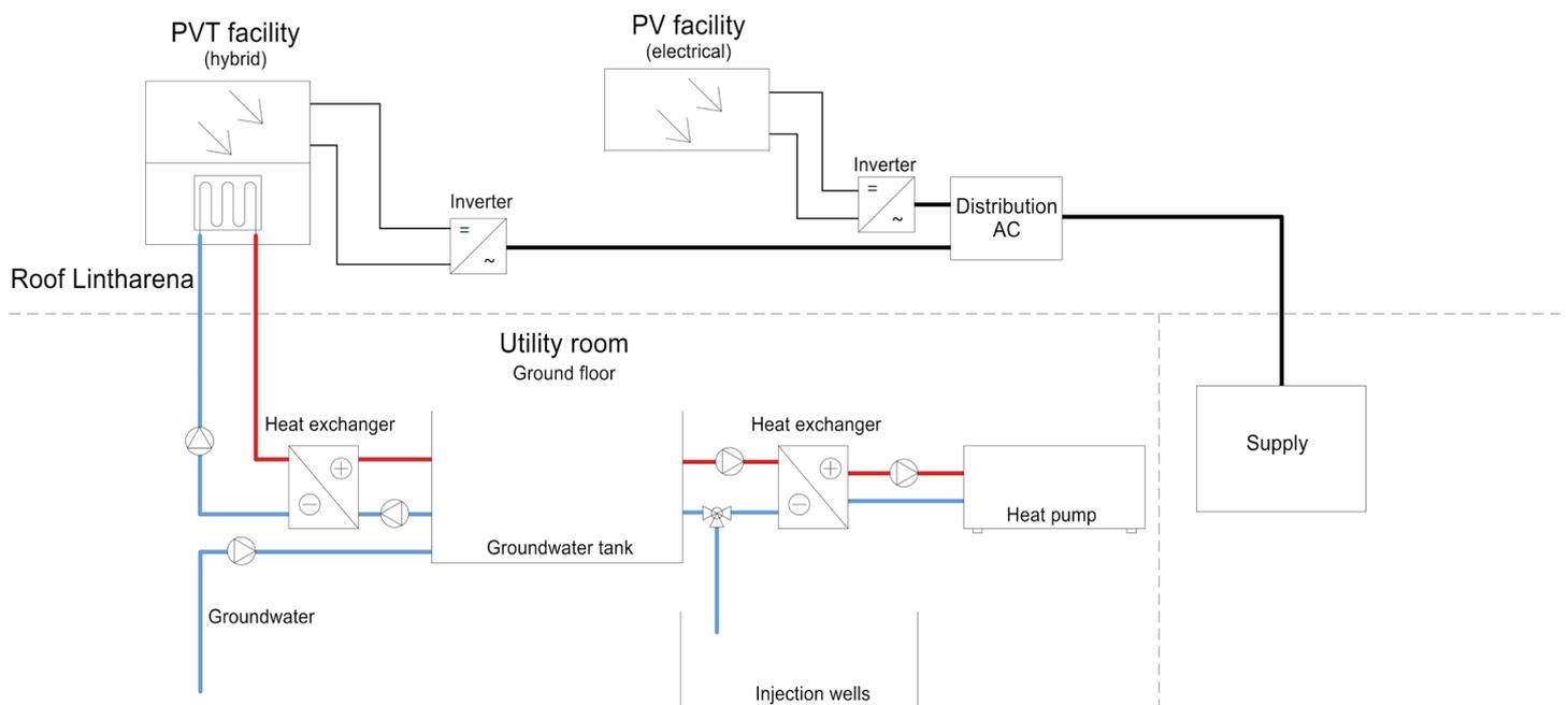
Functional diagram of the solar system on the roof of Lintharena sgu: The electricity from the PV panels (top center) is fed into the grid. The PVT collectors (top left) produce electricity and heat. The heat passes through a heat exchanger in the groundwater tank and is used from there to operate the heat pump. Subsequently, the groundwater in the soil is again supplied via the injection wells. Illustration: ZHAW Wädenswil
