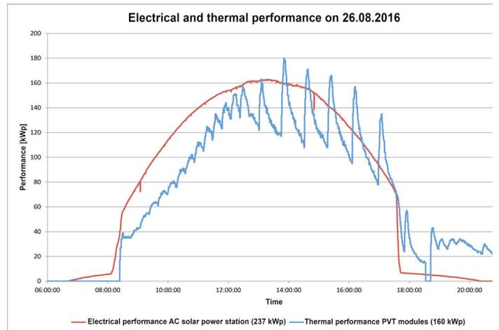
Recording the course of the thermal and electrical performance over a day. The fluctuations of the thermal power supplied by different supply temperatures, which are caused by the operation of the heat pump. Graphic: ZHAW Wädenswil
