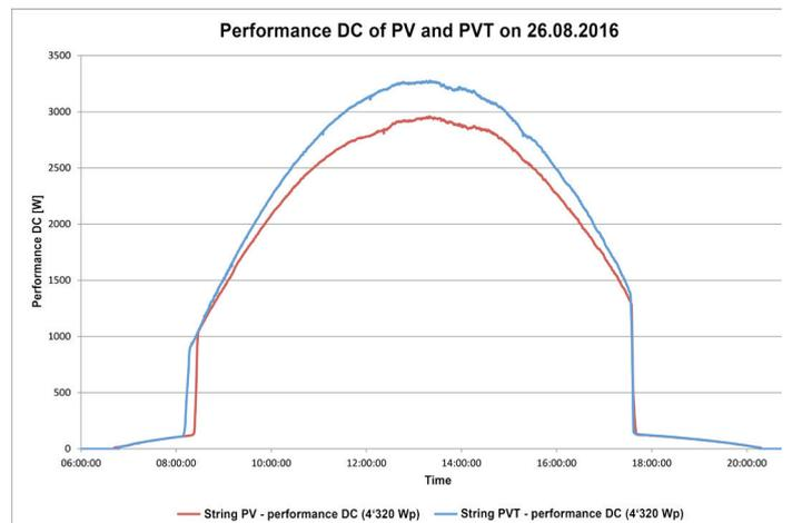
Comparison of DC power between a PV and a PVT cable with the same number of panels and thus the same electric nominal output shows that throughout the day, one fine day in August, the cooling of the PVT panels has a positive effect on performance. The PVT cable produced about 10% more electrical energy than the PV cable. Graphic: ZHAW Wädenswil
