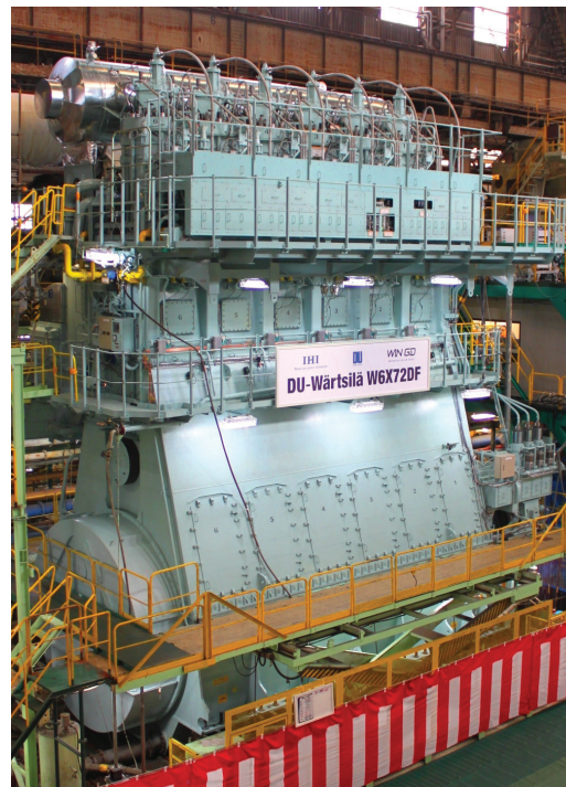
Dual fuel 2-stroke test engine from Win-Gas & Diesel in Winterthur. Photo: WinG&D
