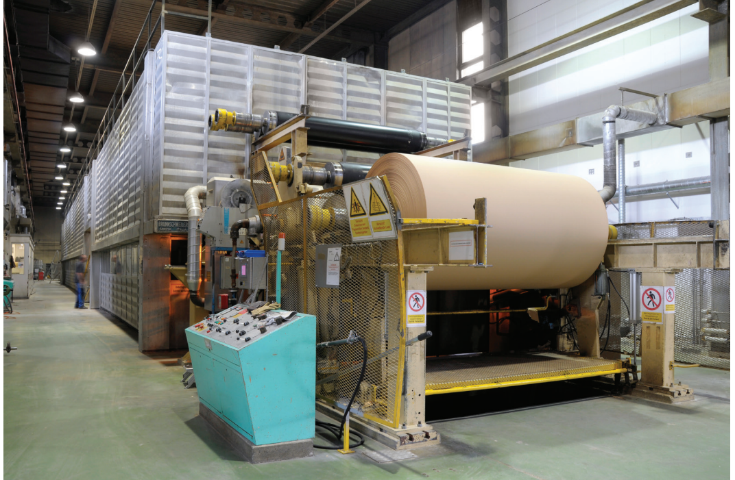
With this system, the Model AG in Weinfelden produces paper rolls, which are later processed into corrugated cardboard. Photo: Model AG
