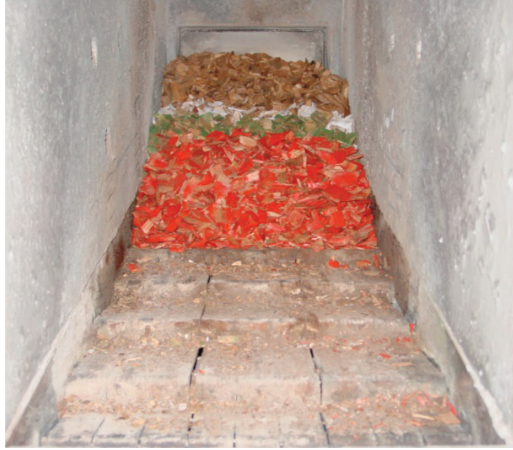
A look into the combustion chamber of a wood-fired heating system (here in the cold state): The chips are placed into the back of the combustion chamber and are transported via the stepped grate forward and in the process, are thermally decomposed by gasification. Left: initial state of superimposed layers of (colored) chips. Right: the final condition after transport by grate movement. Photos: University of Lucerne
