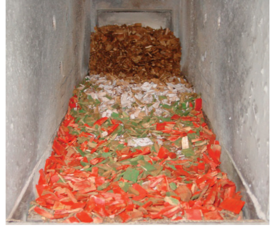
A look into the combustion chamber of a wood-fired heating system (here in the cold state): The chips are placed into the back of the combustion chamber and are transported via the stepped grate forward and in the process, are thermally decomposed by gasification. Left: initial state of superimposed layers of (colored) chips. Right: the final condition after transport by grate movement. Photos: University of Lucerne
