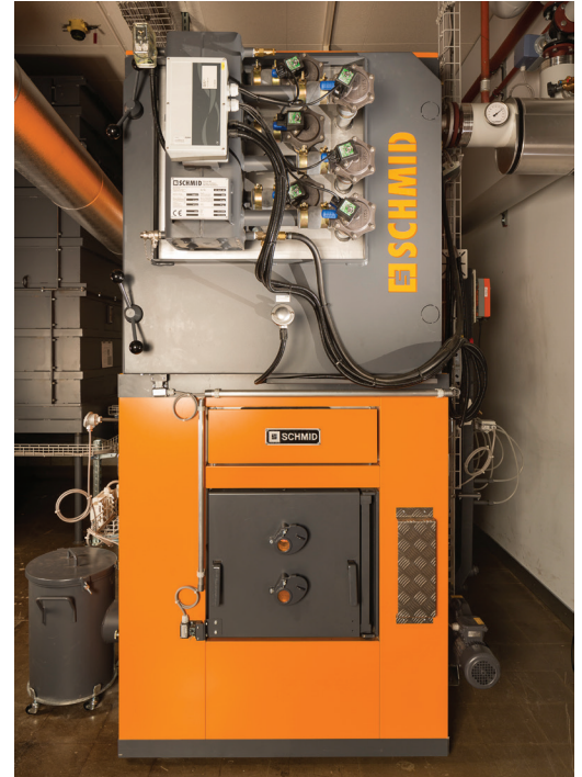
With a test system of 150 kW power capacity, scientists at the University of Lucerne study how to optimize the combustion process in a medium-sized wood-fired heating system. Photo: University of Lucerne
