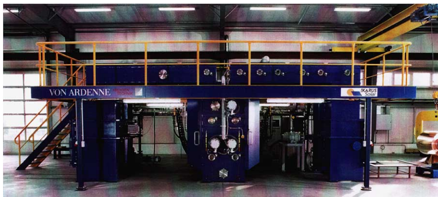
Fig. 9. Industrial thin film deposition equipment for selective absorber coatings on copper sheets based on multilayer a-C:H/Cr nanocomposites. The production capacity is in the order of 2 \times 10^5 \text{ m}^2/\text{year} (IKARUS COATINGS, FRG).
