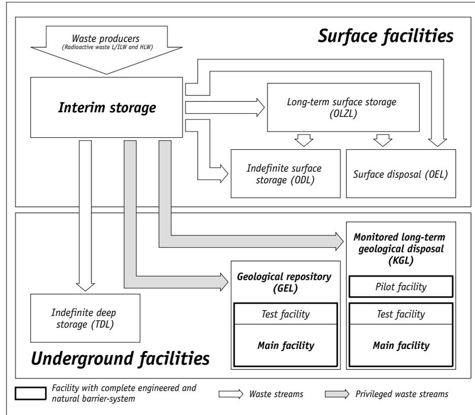
Figure 6: Disposal facilities at the earth's surface (surface facilities) and underground (deep facilities)
