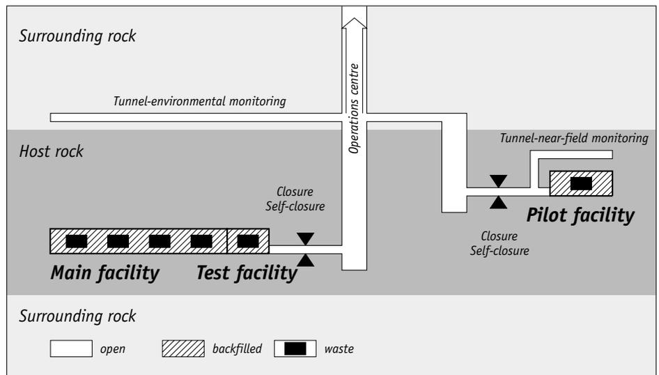
Figure 9: Schematic concept of the monitored long-term geological disposal facility: system elements
