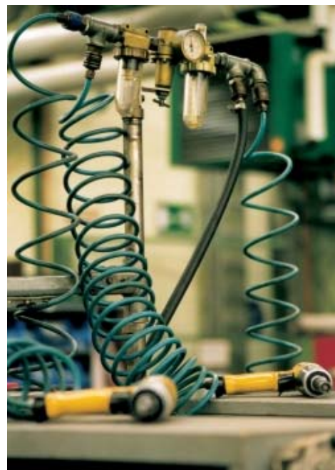
Fig. 3: Energy "gobblers" in compressed air system
