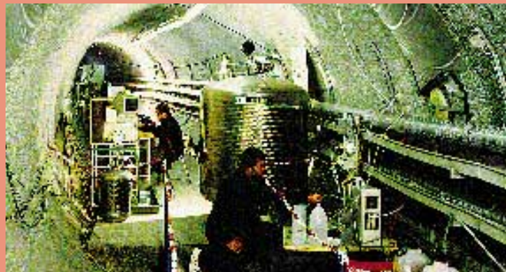
At the field laboratory on the Grimsel Pass, which branches off from a shaft of the hydropower plant, experimental work is carried out with a view to the construction of a final storage site for radioactive waste – in the foreground, a measuring system for the migration of radio-nuclides in rock.
