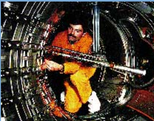
International co-operation on nuclear fusion : coatings with boron carbide developed in Switzerland for the Tokamak interior chamber – shown here inside JET – keep the plasma almost free from impurities.
