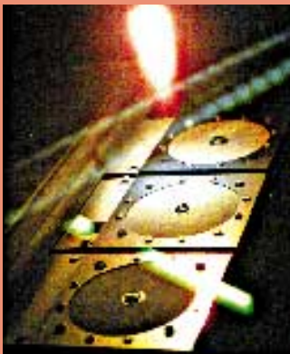
A number of HEXIS membranes each with a diameter of 12 cm are being manufactured simultaneously here using plasma sprays in a vacuum.
