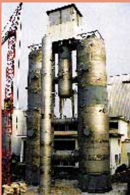
The PANDA test plant at the Paul Scherrer Institute is used to demonstrate the functionality of passive safety systems.
