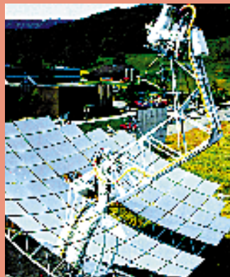
At the focal point of the 90 m 2 parabolic mirror at the Paul Scherrer Institute a cyclone solar reactor is heated by 56 kW of concentrated solar radiation.
