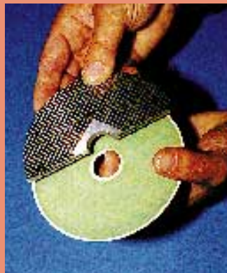
The components of a HEXIS cell: ceramic membrane (green) with electrodes, channelled plate for fuel supply and combustion product draw-off.
