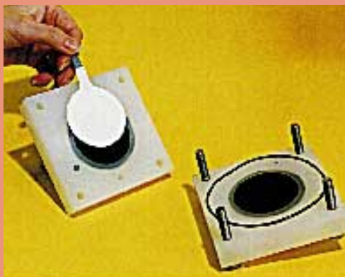
Components of the zinc-air cell: the zinc electrode (hand-held) covered with porous separator material; the dark area (at the right) is the bi-functional air electrode. The thin ring is the seal.
