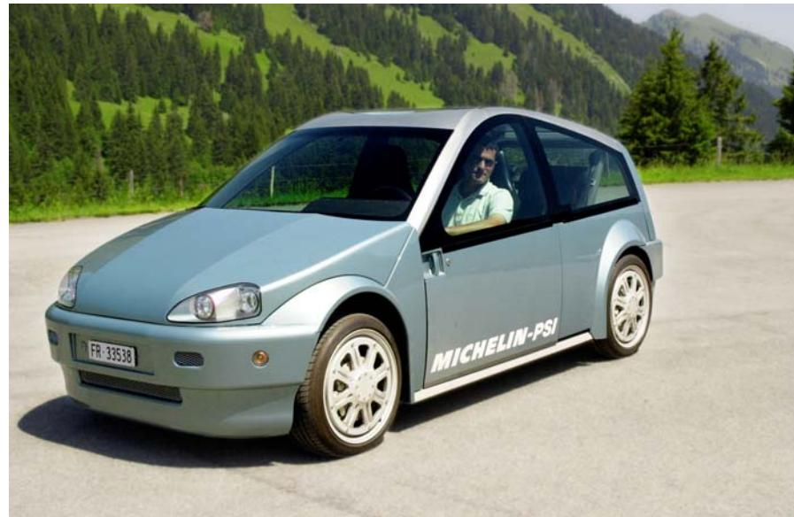
**Power:** 30 kW Fuel Cell Stack, based on H<sub>2</sub> and O<sub>2</sub>
