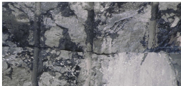
Figure 5. Example of a joint after a shear displacement and dilatancy effect
