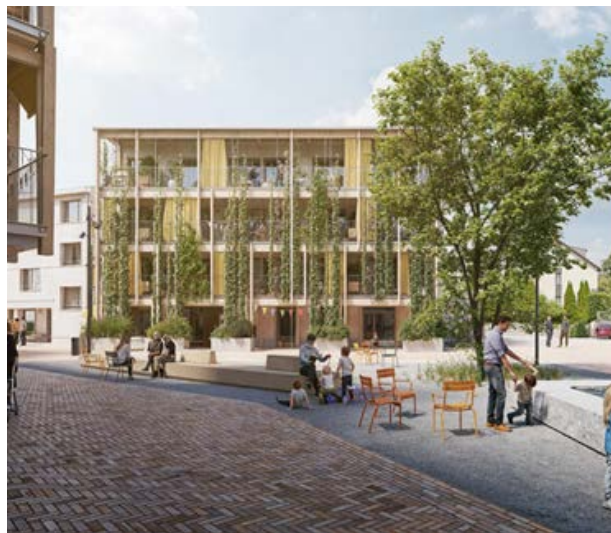
Burkwil housing estate in Meilen: Burkwil offers high-quality, barrier-free flats for around 160 people. The six new buildings were constructed with the lowest possible emissions, using solid timber, clay and low-cement concrete (source: © Tend AG).
