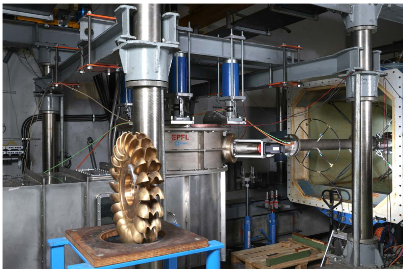
View of the Pelton turbine used for electricity generation (source: final report HydroLEAP, 2025).
