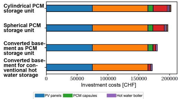
When it comes to the investment costs of an energy system with PV, heat pump, and PCM storage, the latter has the least financial impact. The total cost includes the cost of the underground storage tank (red), the cost of the PCM capsules (green), and the cost of excavation (brown). Added to this is the cost of the hot water boiler (purple). Graphic: Final report HyTES
