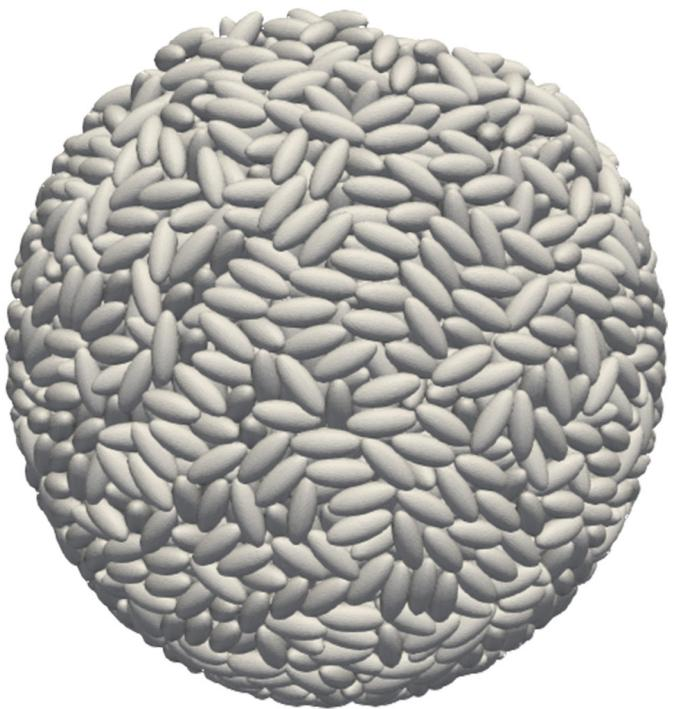
The visualization illustrates two possible storage geometries. The capsules are made of polyethylene plastic and filled with phase change materials. Illustration: HyTES final report
