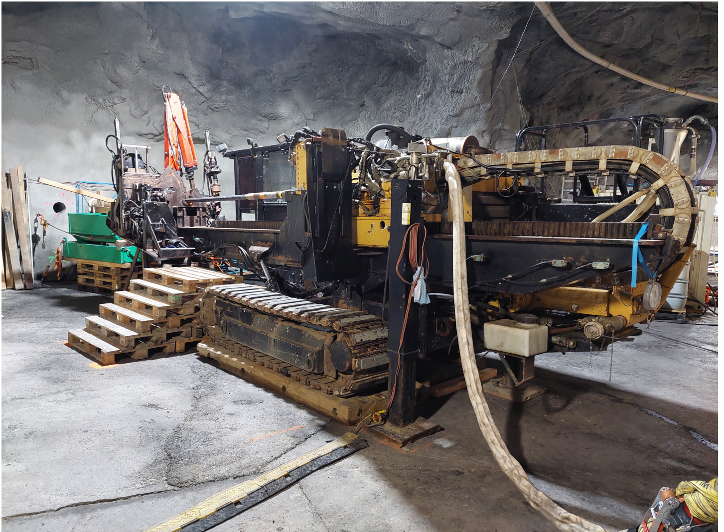
Hagerbach test gallery in the Sarganserland region: DSSD drilling technology was trialled here by driving two 125-metre horizontal boreholes into the mountain, which here consists of limestone (Malm). Photo: ETH Zurich
