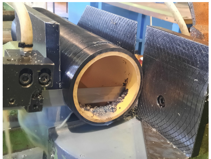
First step of the recycling process: The pressurized storage tank is sawed into pieces. The parts are crushed into chips, which are then heated and compacted. The resulting compound can be molded into any type of part for automotive or appliance applications. Photo: iRAP
