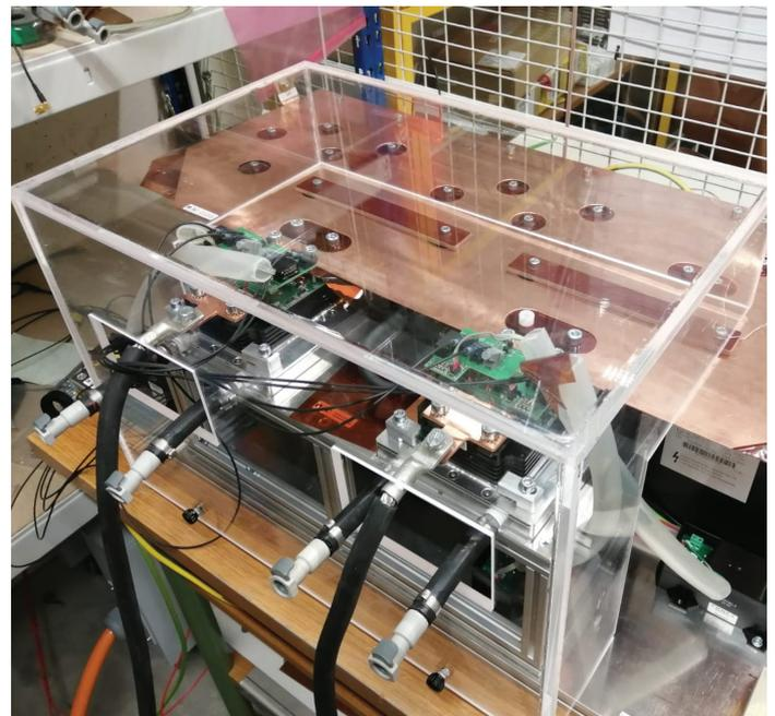
Prototype of a 6.5 kV converter for railroad applications. It contains WBG modules based on SiC from Hitachi Energy Semiconductors. Photo: FHNW
