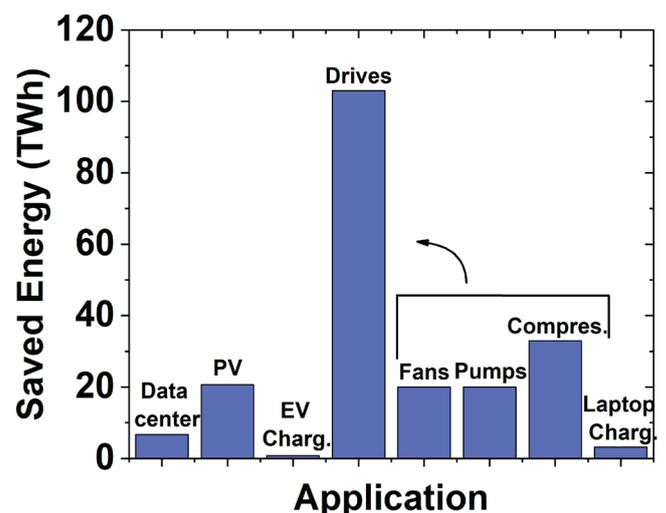
Estimation of the savings that would be achieved if silicon-based converters were replaced by WBG converters in all electrical appliances worldwide (based on the year 2021). The greatest potential lies dormant in the area of electric motors (including electrically powered heating, ventilation and air conditioning systems). Graphic: FHNW
