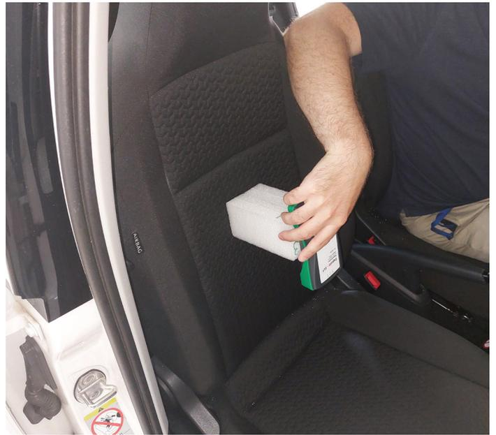
Measuring device for low-frequency magnetic fields on the back seat. Since the strength of EMF fields varies by location, three positions were measured: directly on the backrest, about 5 cm from the backrest, about 10 cm from the backrest (shown). Photo: Fields at Work
