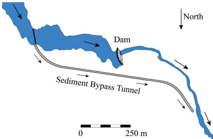
The bypass tunnel begins in the reservoir. Other bypass tunnels take in sediment-laden water already at the inlet of the reservoir, which is very effective, but results in higher construction costs because the tunnel must be longer. Illustration: RESEMO final report
