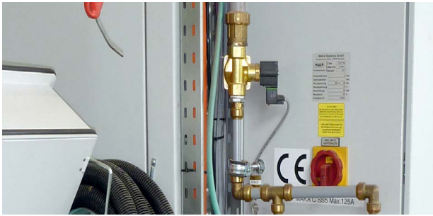
A solenoid valve automatically disconnects a machine from the compressed air network.
