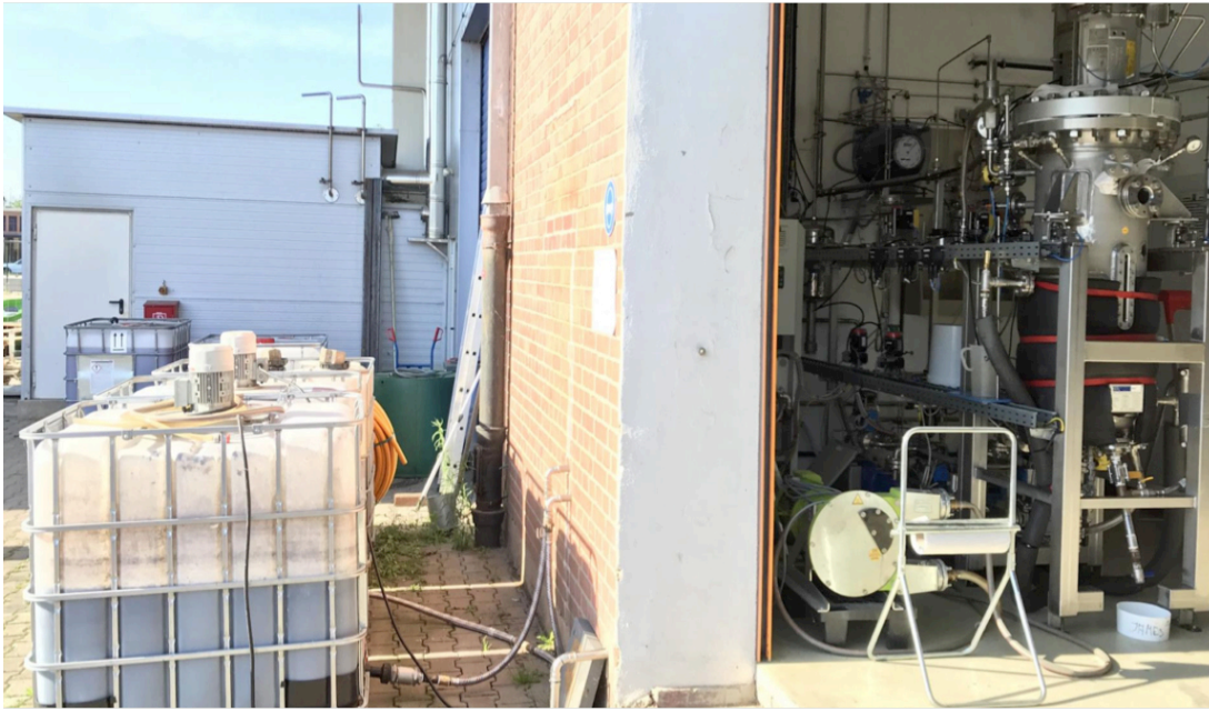
The German company microE-nergy carried out laboratory tests with sewage sludge from the Reinach WWTP. The tests showed that this substrate is suitable for biological methanation. Photo: microE-nergy.
