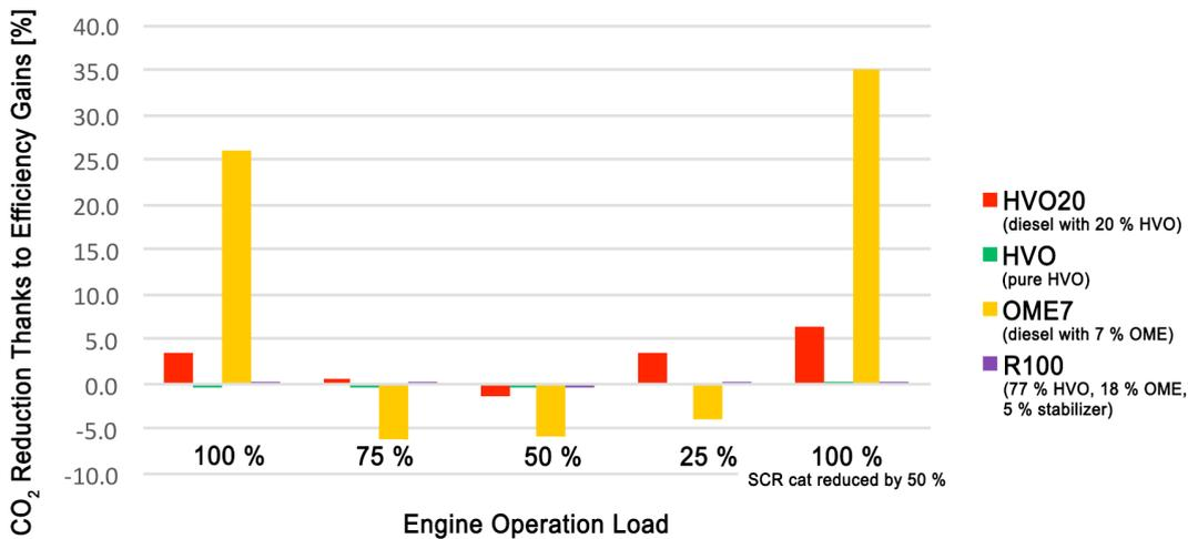
For the pure biofuels (HVO, R100), the additional CO<sub>2</sub> savings are hardly significant due to the efficiency gain. The situation is different for fuel blends containing only a proportion of biofuels (HVO20, OME7).
