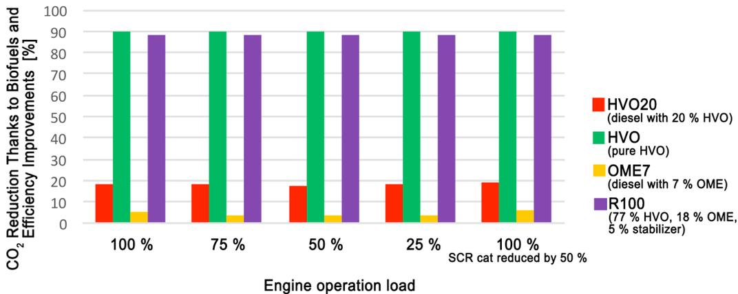
Fuels such as HVO and R100, which are virtually entirely of biogenic origin, can produce around 90% fewer CO<sub>2</sub> emissions than diesel, depending on their origin. In HVO20 and OME7 fuel blends, CO<sub>2</sub> emissions are reduced similarly depending on the proportion of biofuel they contain. Graphic: Final report ReVerDi/edited B. Vogel
