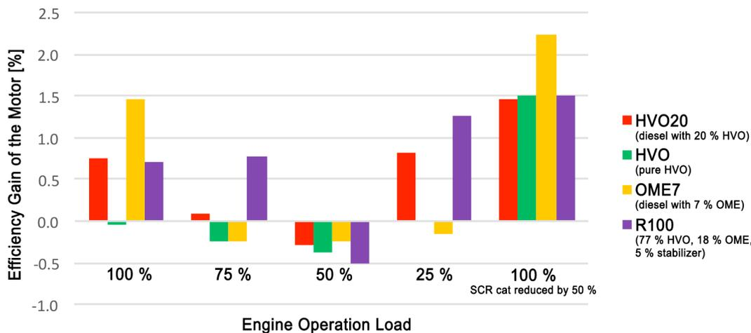
Since biofuels are less prone to form soot, they place less strain on the soot particle filter. The energy saved in this way can be converted into efficiency gains of the drive energy. Depending on the fuel or fuel mixture, this amounts to a good two percent. Graphic: Final report ReVerDi/edited B. Vogel
