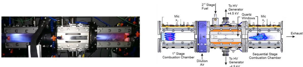
Figure 1: Atmospheric pressure sequential combustor.
