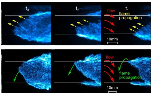
Two distinct flame propagation pathways in a gas turbine burner: (a) 50° (b) 65° Swirler
