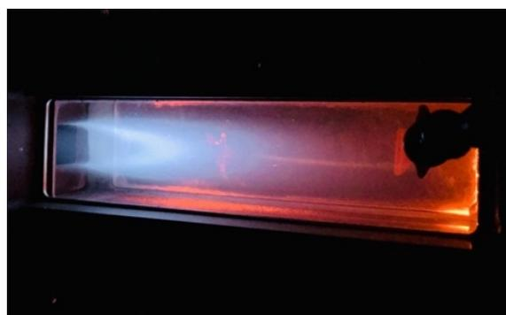
Combustion of Hydrogen in the hot vitiated flow of a laboratory sequential combustor
