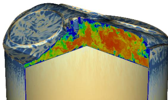
DNS of full scale pent-roof engine: temperature distribution on cut planes, wall heat flux on surfaces
