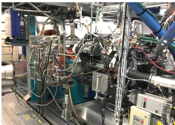
6-cylinder Diesel-Engine on a test rig with DME injection and EGR blower
