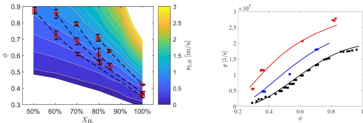
Figure 1: On the left, the flashback limits at  $p=2.5$  bar and  $T_{pre}=200$  °C [1]. On the right, experimentally measured boundary layer flashback limit data of Eichler [2] (squares) compared to the model developed in this work (lines). The flashback limits cover three discrete preheat temperatures of 20 °C (black), 200 °C (blue), and 400 °C (red).
