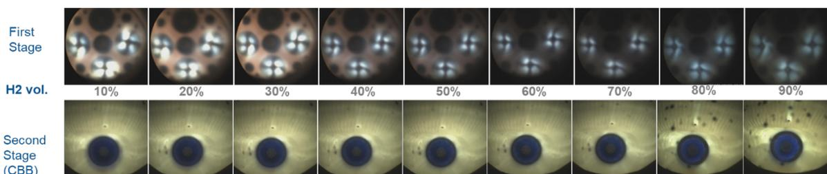
**Operation concept for highly reactive fuels (hydrogen): the first stage flame temperature is tuned for optimum boundary conditions of the second stage (Center Body Burner), maintaining maximum combustor exit temperature for best engine performance at low NO<sub>x</sub> emissions. Images from full-scale high-pressure testing.**
