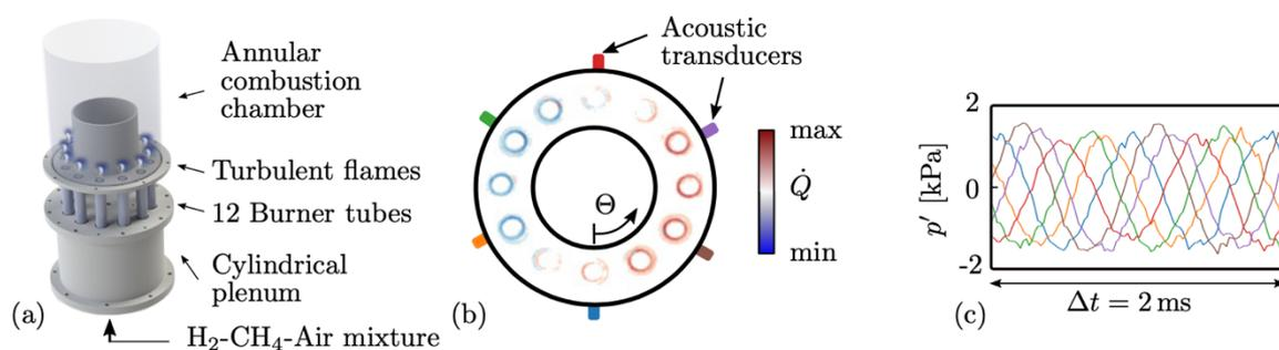
Figure 1: (a) Model gas turbine combustor. (b) Phase-averaged flame chemiluminescence. (c) Acoustic pressure recorded with 6 transducers. During the selected interval, the thermoacoustic limit-cycle is a quasi-purely spinning eigenmode.
