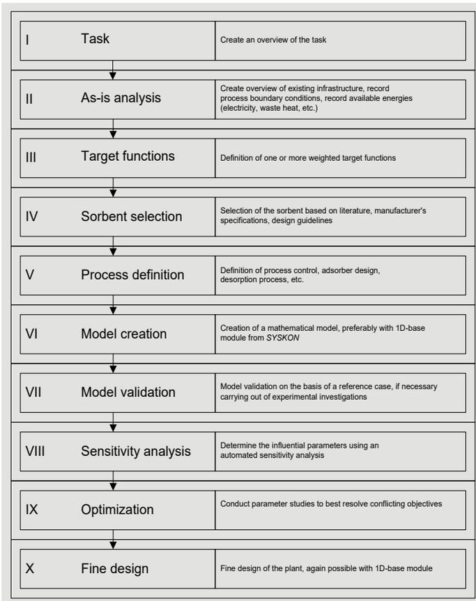
In order to optimally design adsorption processes from the gas phase, HSLU researchers have developed a guideline with ten steps. Illustration: Guide EESP
