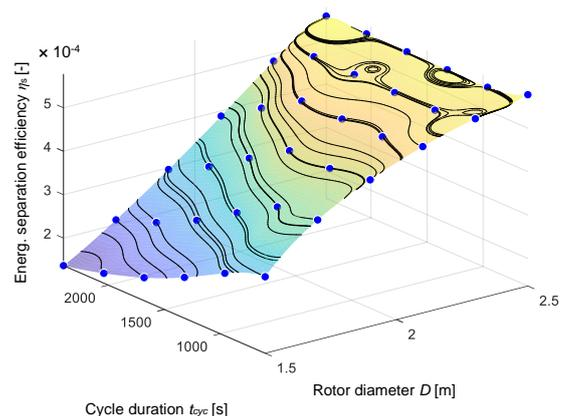
This diagram illustrates three important parameters of gas purification by adsorption. From the diagram one can see, for example, that the rotor diameter in this example must be chosen as large as possible and the cycle duration as short as possible in order to achieve a high energetic separation efficiency. The desired objectives can be achieved by suitable mathematical analysis (Pareto-optimization). Illustration: Final report EESP
