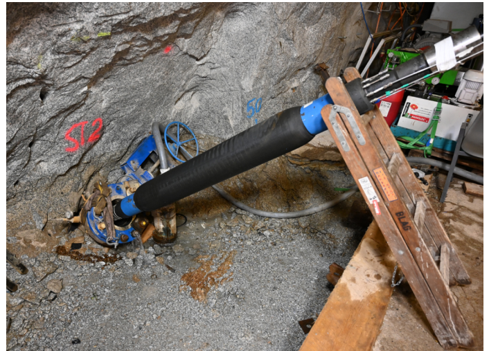
A packer is inserted into the borehole. A packer is an inflatable rubber sleeve (visible in the photo between the two blue pipe sections). This divides the borehole into individual zones. Packers are subjected to pressures up to 200 bar during the tests. Graphic: Geo-Energie Suisse
