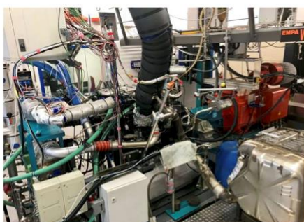
“Diesel engine test rig with EGR blower” G. Hardy / FPT et. P. Soltic / Empa
