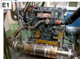
Test engine (E1) Liebherr D934S on the engine dynamometer
