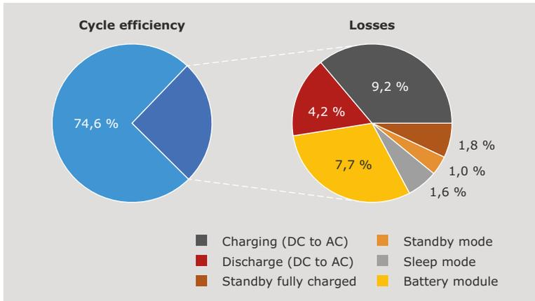
Test result of an alternating current (AC) coupled battery home storage system. A new test procedure from the OST University of Applied Sciences examines batteries in a 3-day test profile that covers all typical operating conditions for the battery. It provides reproducible key figures on the efficiency of the systems under different control approaches such as self-consumption, electricity price and grid use, and indicates at what points losses occur (source: OST-SPF).
