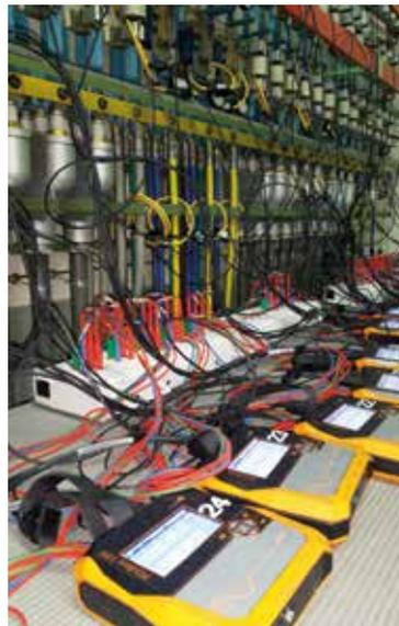
A large number of different influencing parameters make it difficult to compare power quality (PQ) across grids. As part of various measurement campaigns, a PQ index was developed that enables the evaluation of different PQ phenomena using a single key figure (source: Bern University of Applied Sciences BFH).
