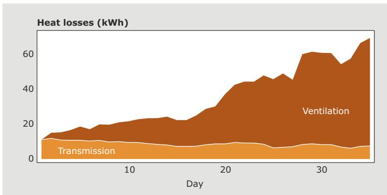
Only about 25% of heat loss occurs through transmission (heat dissipation via the building envelope), the rest is at the expense of constant ventilation. More energy can be saved through heat recovery technology than through insulation of the building envelope.
