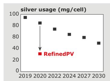
Silver consumption for silicon solar cells (monofacial, p-type) according to the International Technology Roadmap for Photovoltaic (ITRPV, 2020).
