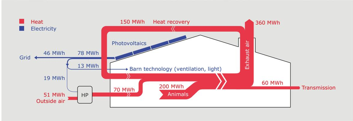
(Top) The Leuenberger fattening poultry house, Hellsau BE, 2019. (Bottom) Energy flow diagram for heat and electricity in a Minergie poultry farm (Data Hellsau).
