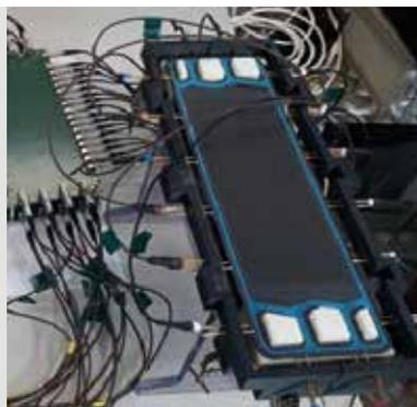
(Left) In order to examine the conductivity distribution  $\sigma$  in fuel cells by electrical impedance tomography, an alternating current  $I$  is applied between two electrodes (red) and the resulting changes in the surface potential are measured between pairs of electrodes. Repetition with many different configurations provides data from which the conductivity distribution in the membrane can be calculated. (Right) Experimental setup at the Paul Scherrer Institute.
