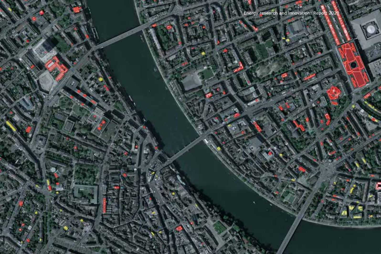
With machine learning, solar plants can be identified in aerial photographs. The result here shows a section of the city of Basel with photovoltaic installations marked in red and solar thermal installations marked in yellow.
