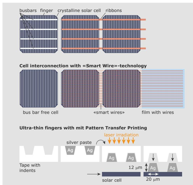
To contact crystalline silicon solar cells, metallic fingers and busbars are printed on the cells as current busbars. In recent years, technologies have been developed to connect cells without busbars and to reduce the width of the contact fingers. Both help to improve performance, as the cell is less shaded and there is less ohmic loss. Furthermore, silver is massively saved, which is a relevant cost factor.
