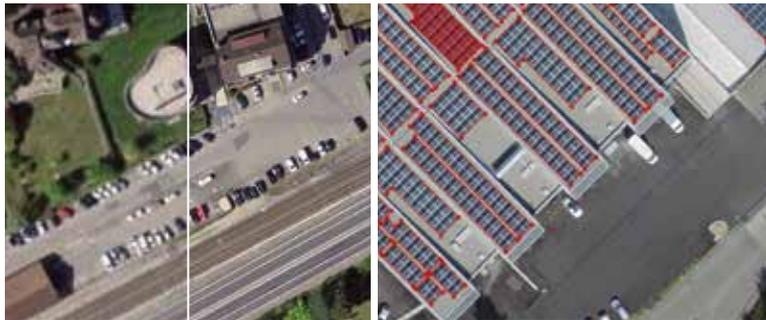
A decisive prerequisite for the identification of solar installations on aerial photographs is a correspondingly high resolution. The Federal Office of Topography swisstopo now provides images with a resolution of 10 cm. The left image illustrates this in comparison to the previous resolution of 25 cm (left part of the image). In order to train the neural network, a total of 7,839 images were prepared where photovoltaic and thermal plants were marked with polygons (source: FHNW).
