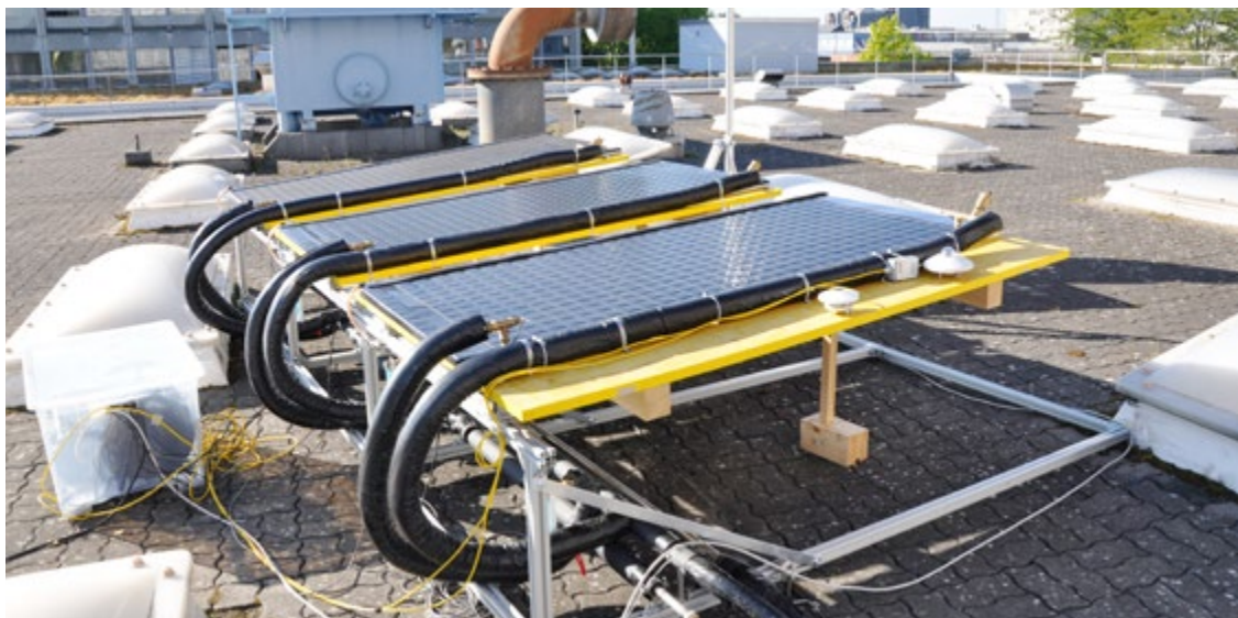
Test bench measurements to determine the cooling capacity of three solar absorbers as part of the project "Heating and cooling via thermally activated external surfaces" at the FHNW. The uncovered solar absorbers function as external heat exchangers that can absorb heat from the environment and by absorbing solar radiation in the heating mode. During the cooling mode at night, they give off heat to the environment. © FHNW IEBau
