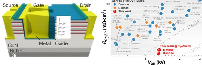
Figure 1. (left) Schematic of the multichannel slanted tri-gate MOSHEMTs. (right)  $R_{on,SP}$  versus  $V_{BR}$  benchmarks of multi-channel MOSHEMTs against conventional single-channel GaN (MOS)HEMTs in the literature, showing a substantial improvement by the multi-channel power devices.
