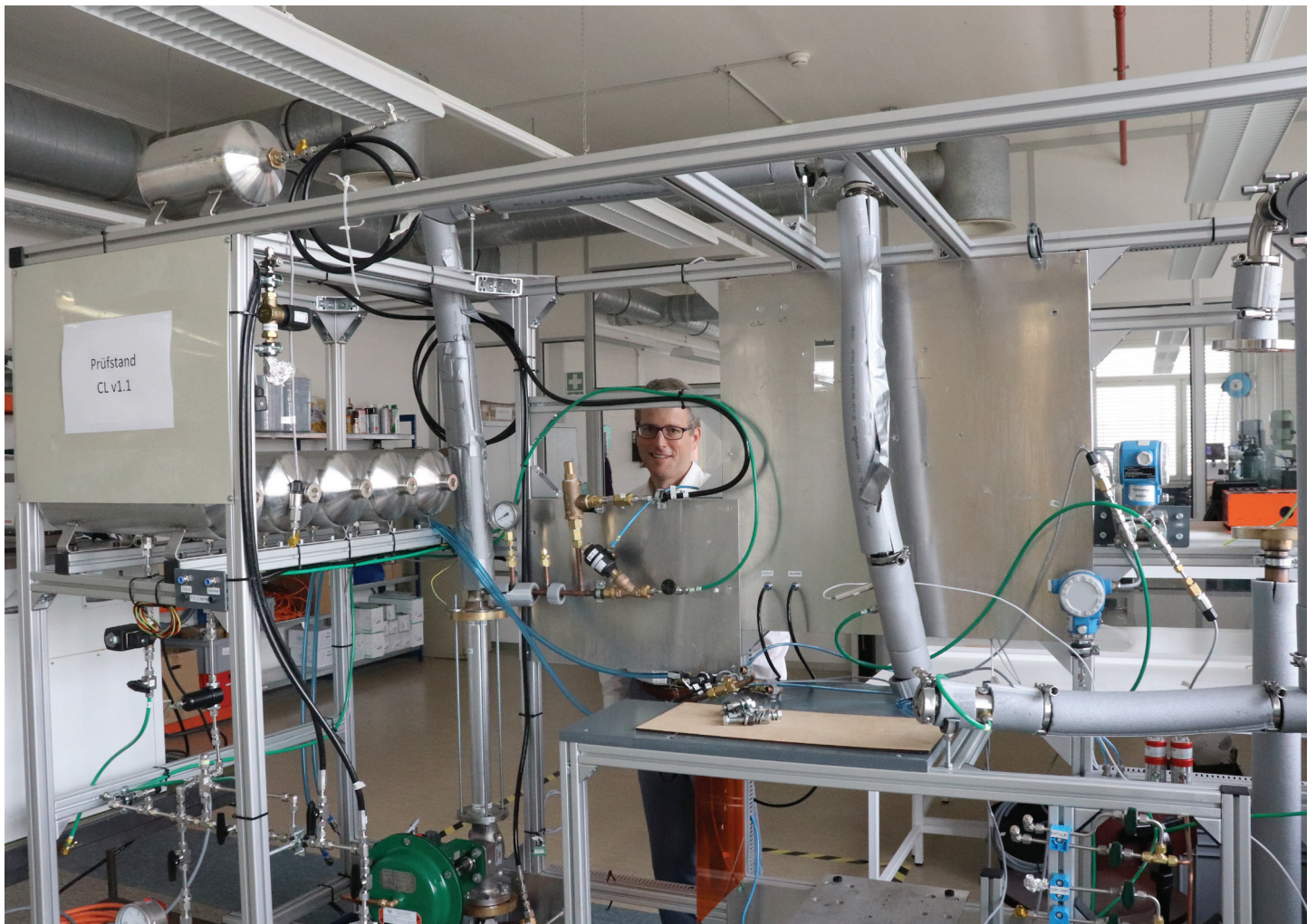
Martin Bartholet shows one of the test benches used by Celeroton engineers to test the operating behavior of turbo compressors. Photo: B. Vogel
