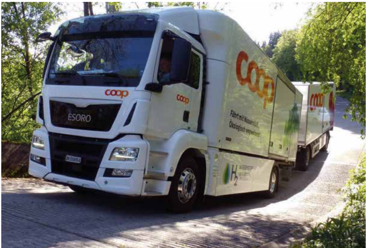
Prototype fuel cell truck developed by Esoro in cooperation with Swiss Hydrogen: Successful drive-off test at a slope of 30 % and a total weight (truck plus trailer) of 35 tons (source: Esoro).
