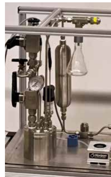
(Right) Laboratory prototype of an aluminium converter for hydrogen production in combination with a 12 W fuel cell (source: SPF).
