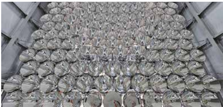
(Top) Novel solar receiver concept from the company Synhelion with radiative heat transfer (graphics after Synhelion). (Upper left) A 200 kW pilot reactor (source: Synhelion) was successfully tested in 2019 on the solar simulator of the German Aerospace Center (lower left, source/credit: DLR/M. Hauschild) and temperatures of over 1550 °C were reached.
