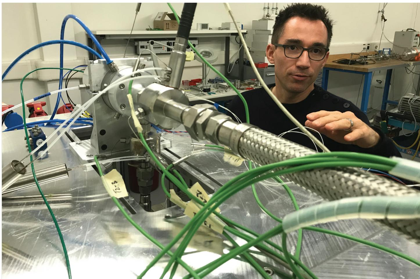
Prof. Jürg Schiffmann shows the test bench in the laboratory, on which the oil-free radial compressor can be tested as a component of a heat pump circuit. Photo: B. Vogel
