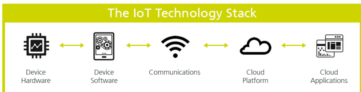
Figure 3: The five layers of the IoT technology stack (image from Elizalde, s.a. [2015]).
