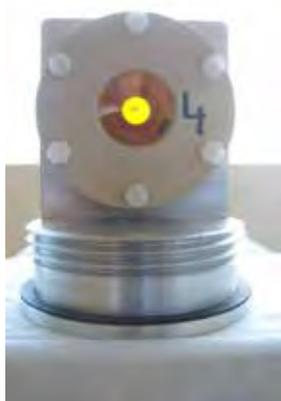
Figure 2: SLS sample holder with a small strip in the center containing fuel particles
