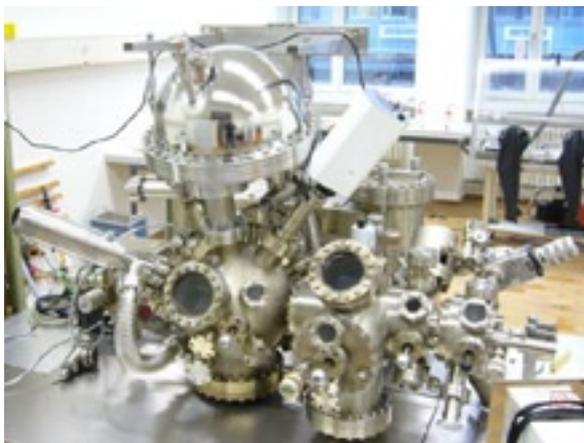
Figur 15: Electron Spectroscopy for Chemical Analysis (ESCA) Set-up an der EMPA [17]
