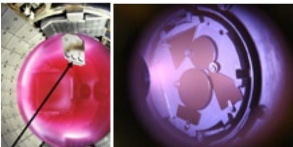
**Figure 2:** left: Rhodium mirrors exposed in a fusion reactor; right: Rhodium mirrors deposition (picture University of Basle).
