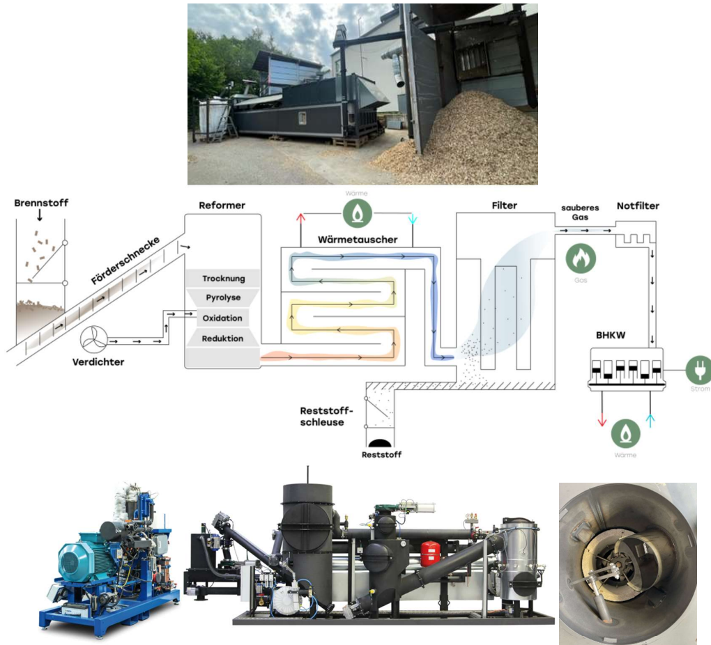
Figure 4.9: Gasifier CHP module from Spanner Re 2 . Top: Dryer. Middle: plant layout. Bottom: new plant before delivery. Source: https://re2.energy/de/ and [18]. Photos top and bottom right: T. Nussbaumer, 2024.
