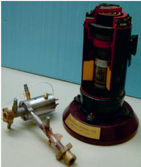
*Figure 3: Size comparison between traditional scroll compressor (right) and high-speed micro centrifugal compressor with equivalent capacity and efficiency (left)*
