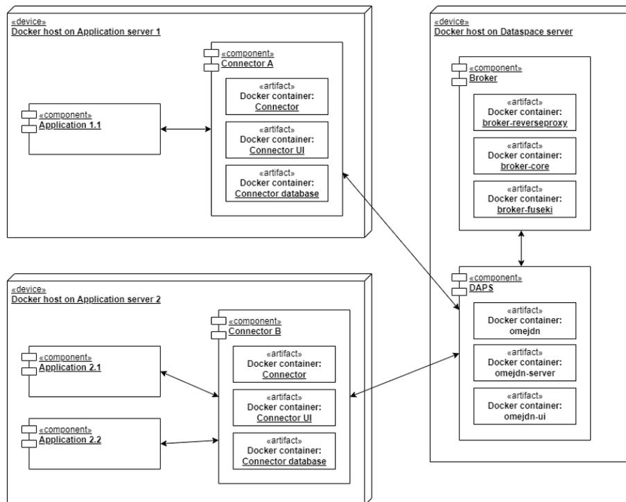
**Figure 9 General deployment diagram for a data space that can be reached from public internet**
