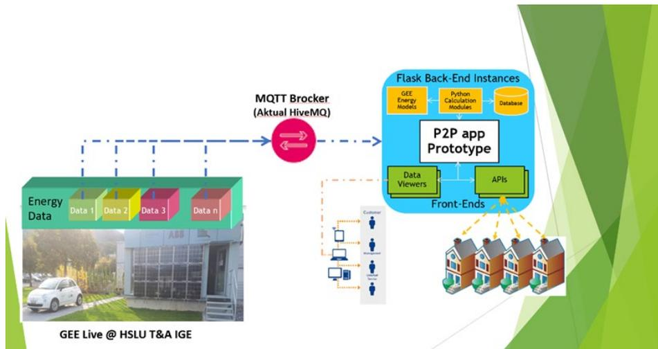
Figure 30 Architecture of P2P software framework (demo)
