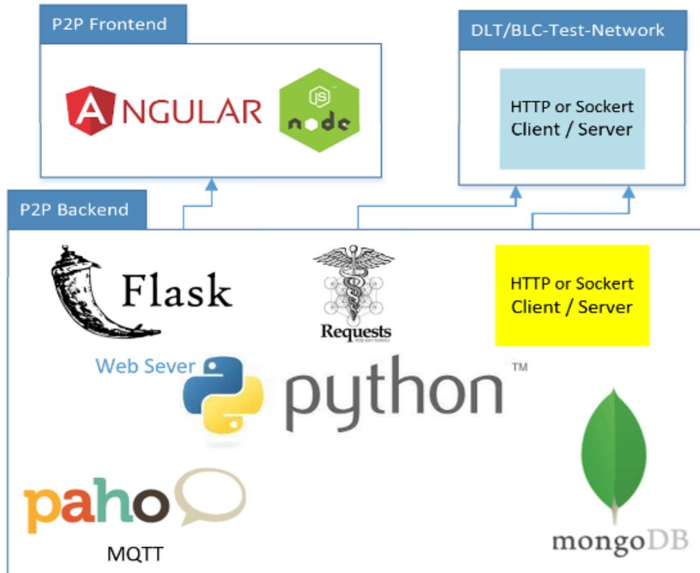
Figure 31 Software stack used for the front- and back-end of the P2P demo
