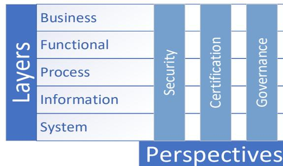
**Figure 6 The five layers and three perspectives of the reference architecture model of international data spaces**
