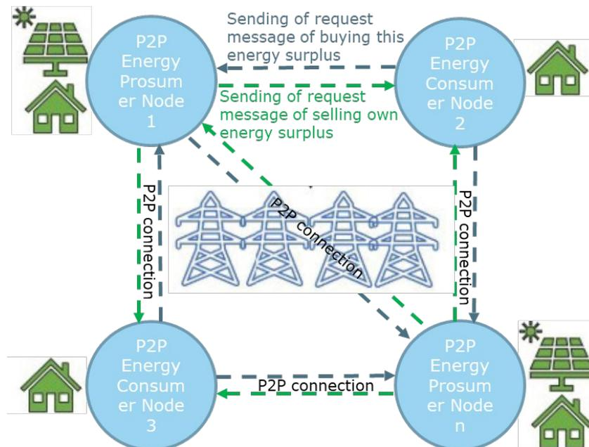
**Figure 28 Structure of P2P connections**
