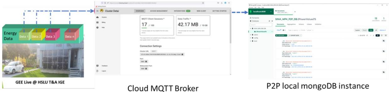
**Figure 44 Energy dataflows from GEE to target P2P software framework**
