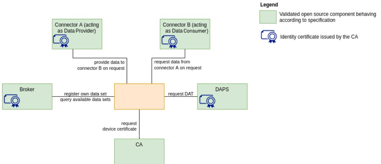
**Figure 7** The components of a minimum viable data space with the component under test in the center. CA and DAPS form the Identity Provider. Source: IDSA (2022b)
