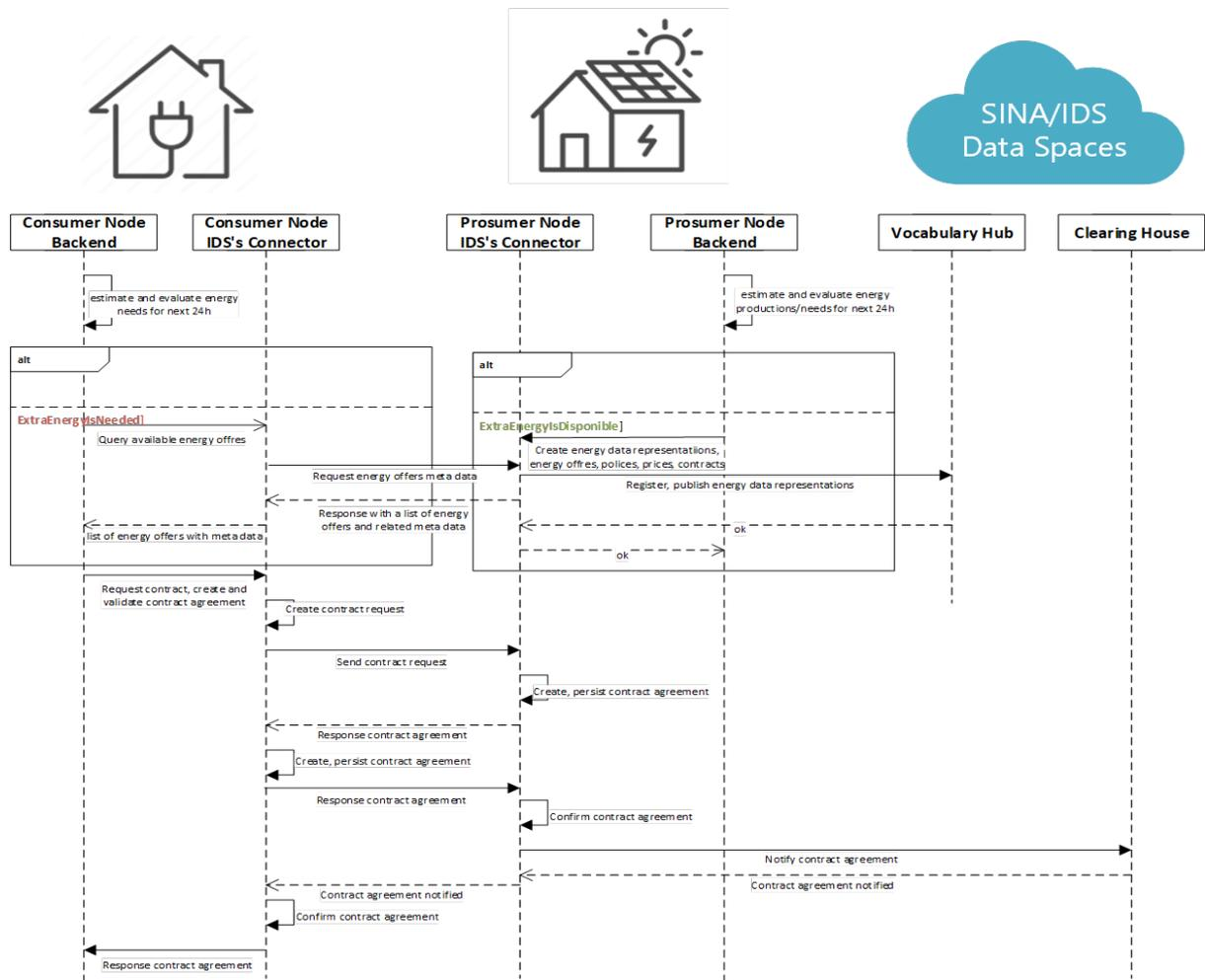
**Figure 32 Sequence diagram of data interactions between P2P nodes**
