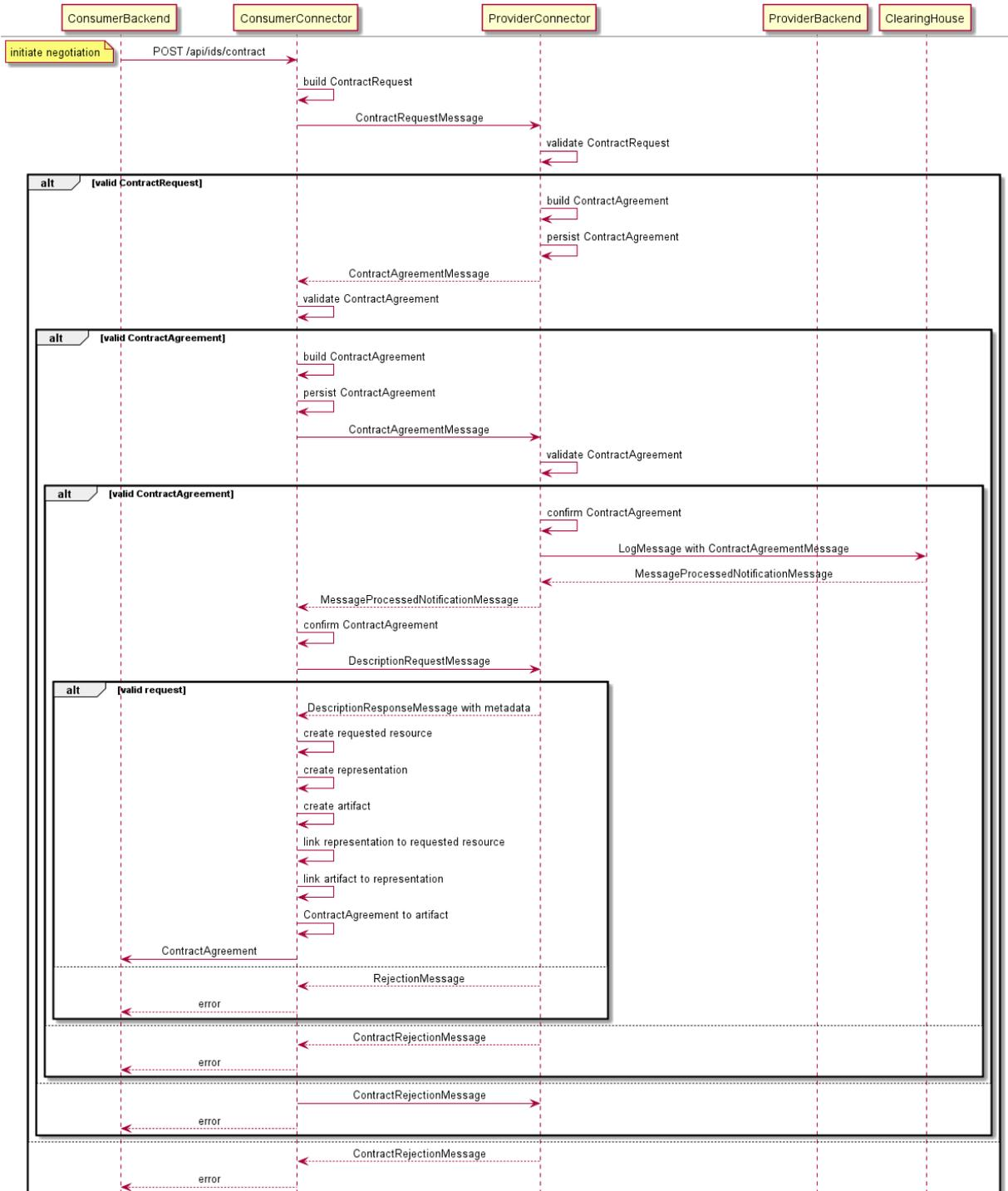
Figure 13 Contract negotiation process for consumer and provider. Source: Fraunhofer ISST (2021)
