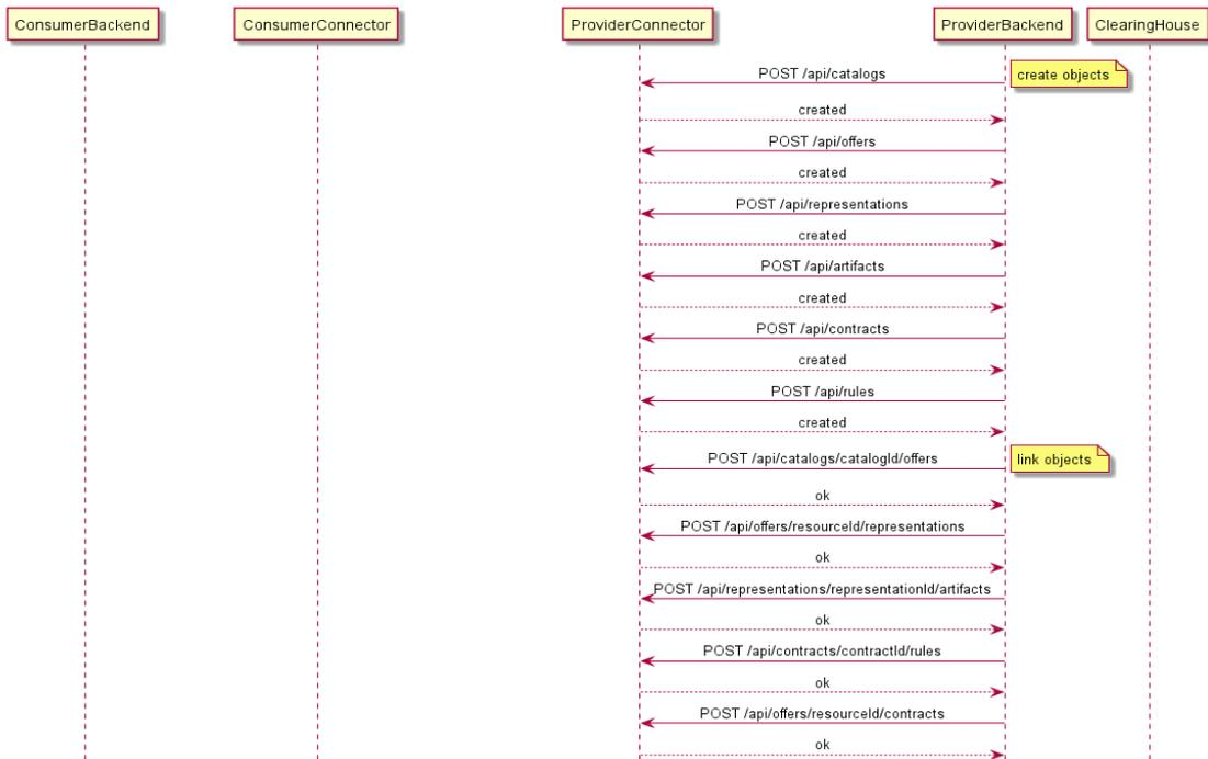
Figure 11 Preparation work needed by data provider for the exchange of data. Source: Fraunhofer ISST (2021)
