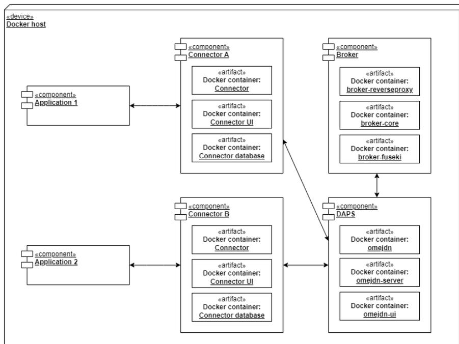
**Figure 8** General deployment diagram for the minimum viable data space that is used as a base for the demonstration of the SINA data space running in a local network
