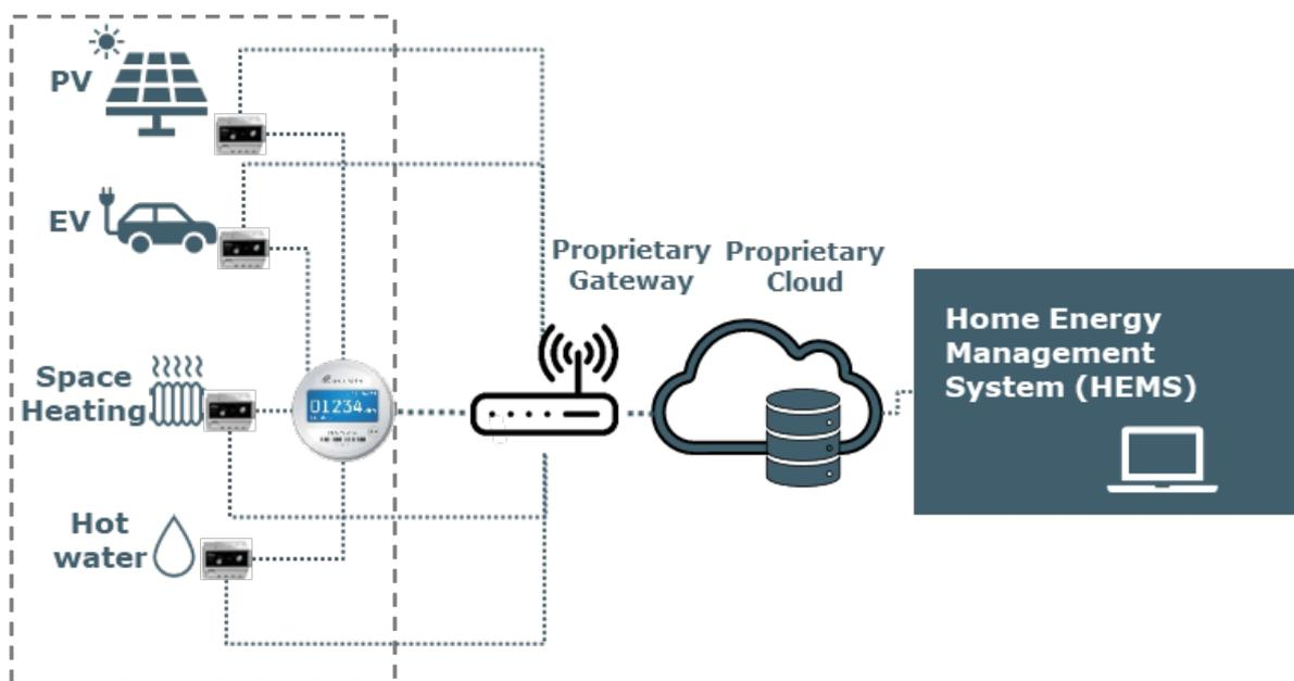
**Figure 3 Conventional set-up with the application of home energy management system (HEMS)**
