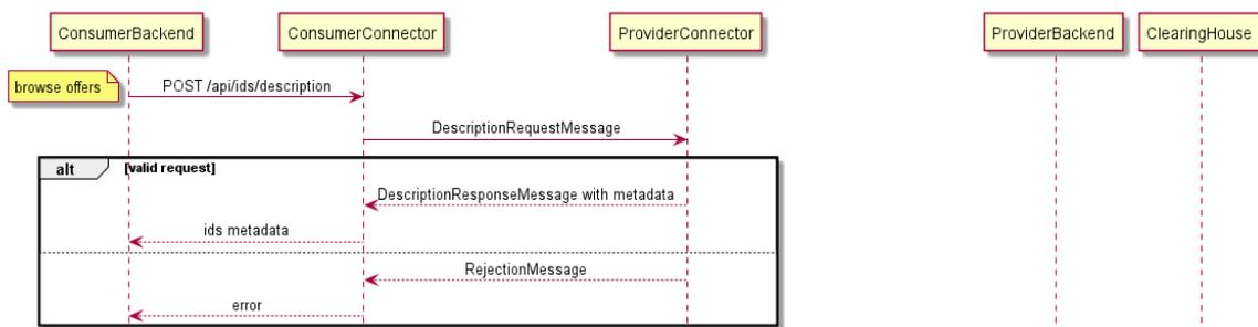
Figure 12 Process for the consumer to browse for offers from a provider. Source: Fraunhofer ISST (2021)
