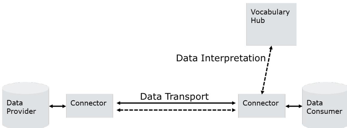
**Figure 16 Representation of interaction between data space connector and vocabulary hub**
