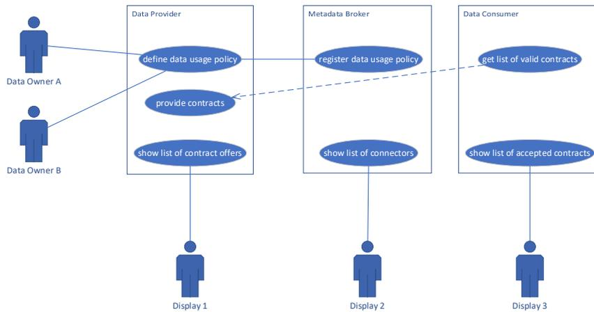
**Figure 15 The use case diagram showing the perspective of offers and contracts and how they are registered and listed in the demonstrator**
