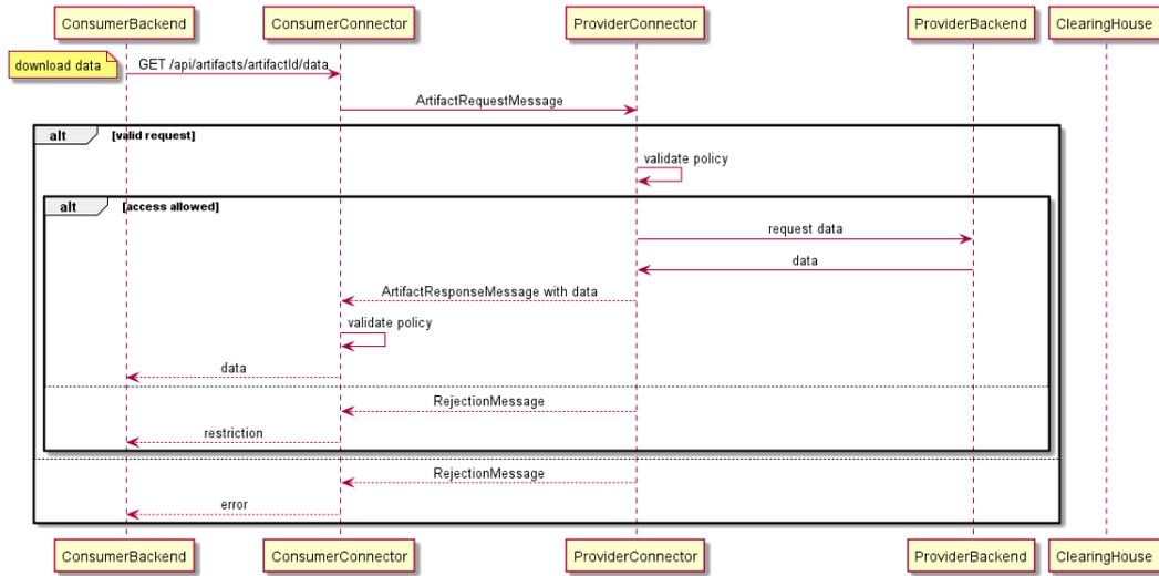
**Figure 14 Data exchange process which is only possible when a contract is accepted from both sides. Source: Fraunhofer ISST (2021)**
