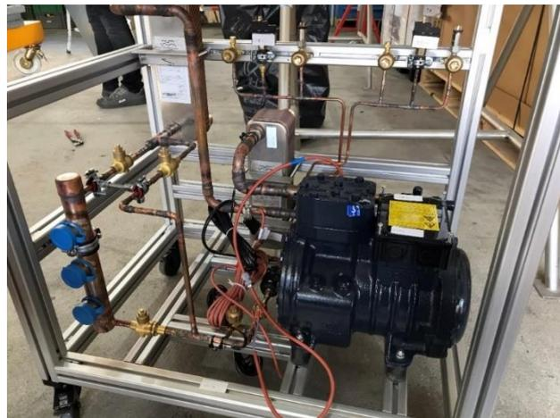
Figure 3: 3D drawing of the HP with overall dimensions and picture of the refrigeration circuit without thermal insulation (source: ZERO-C).
