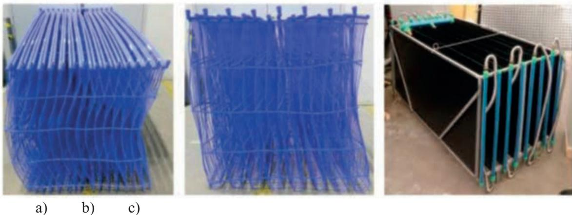
**Figure 3: Examples of heat exchangers (a) 16 S-type capillary mats (b) 8 G-type capillary mats and (c) 8 polypropylene flat plates.**
